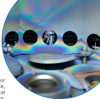
The SYRUSpro 710 machine is a physical vapor deposition machine with advanced plasma source, allowing the fabrication of high performances optical interference filters and microstructured components. Two systems are available allowing to cover a wide range of possible deposited materials including oxydes, metals or chalchogenides. Accurate control of their optical properties is possible thanks to dedicated optical monitoring systems.
