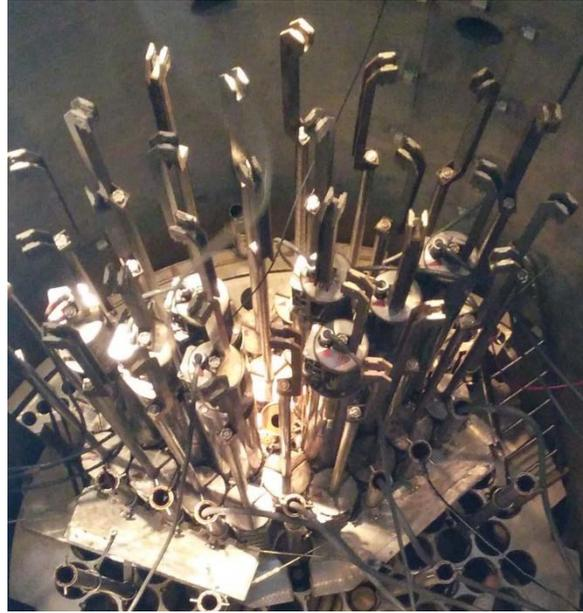
Figure 6.10. Photo of the radial section of VVER-1000 transport Mock-Up at LR-0 [Kostal 2016].
