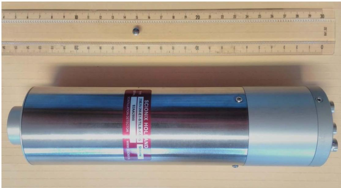
**Figure 5.23.** 25.4 mm  $\times$  25.4 mm ortho-cylindrical solution-grown stilbene detector (plus PMT).
