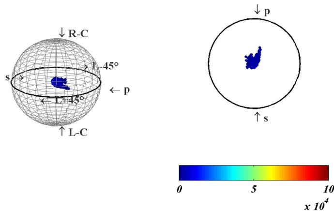
Fig. 9. Polarization states on the Poincaré sphere for the polished surface sample (S<sub>3</sub>). Unpolarized illumination.
