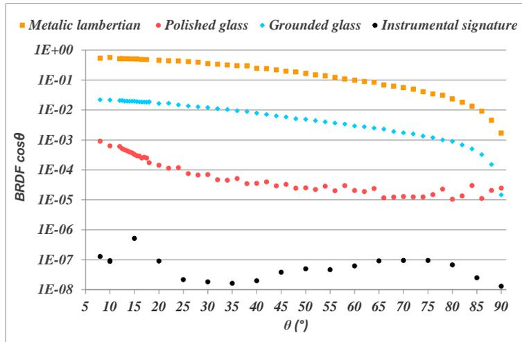
Fig. 2. Angle-resolved scattering curves (ARS) of the surface samples in Fig. 1.
