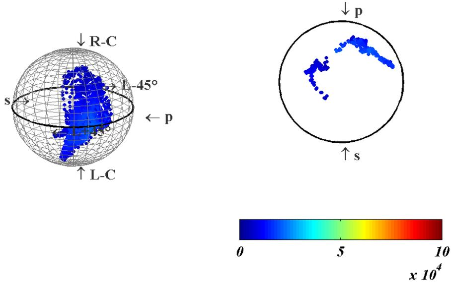
Fig. 18. Polarization states for the bulk grey sample- unpolarized illumination.
