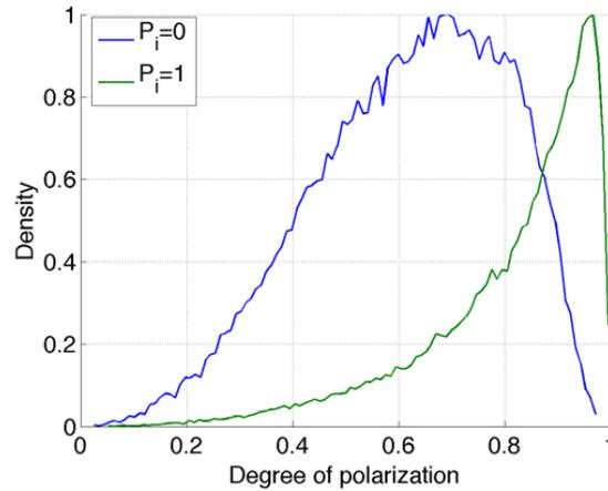
Fig. 20. pdf of the polarization degree calculated for a bulk sample under polarized (green curve) and un-polarized (blue curve) illumination.
