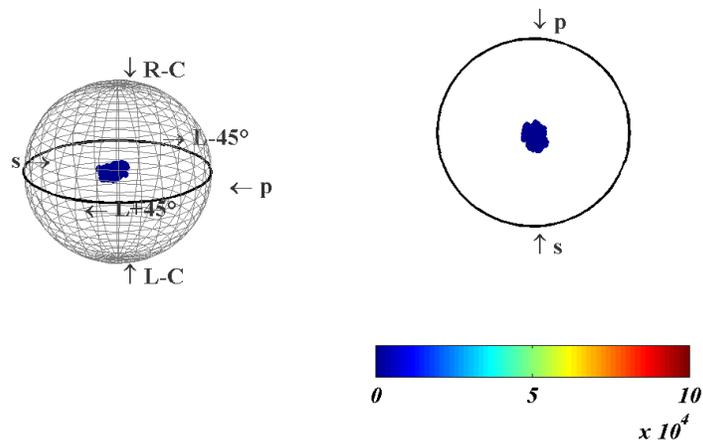
Fig. 7. Polarization states on the Poincaré sphere for the Au lambertian surface sample (S<sub>1</sub>). Unpolarized illumination.
