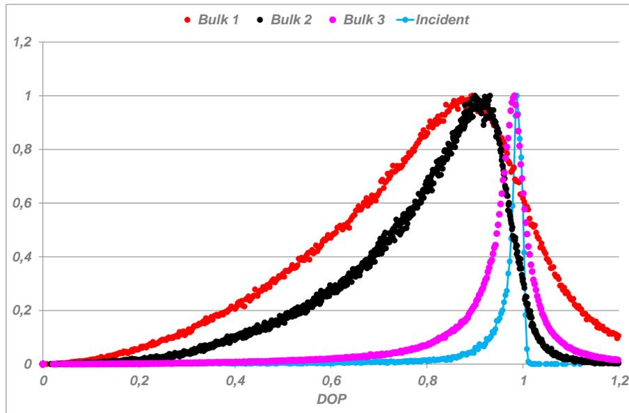
Fig. 12. Normalized dop histograms of the 3 bulk samples -Polarized illumination. B<sub>1</sub>: white bulk, B<sub>2</sub>: grey bulk, B<sub>3</sub>: black bulk.
