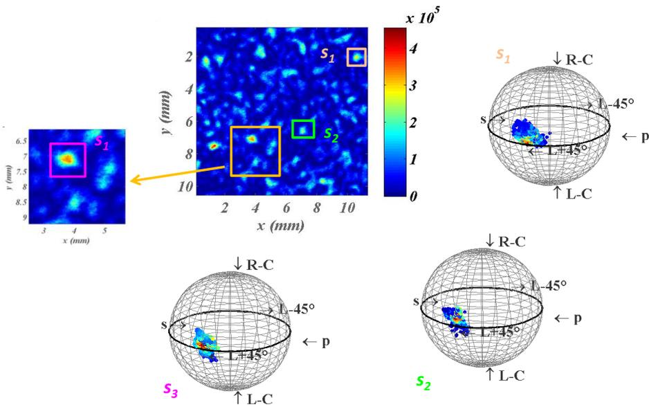
Fig. 4. Polarization states on the Poincaré sphere for the Au lambertian sample ( $S_1$ )- Polarized illumination.
