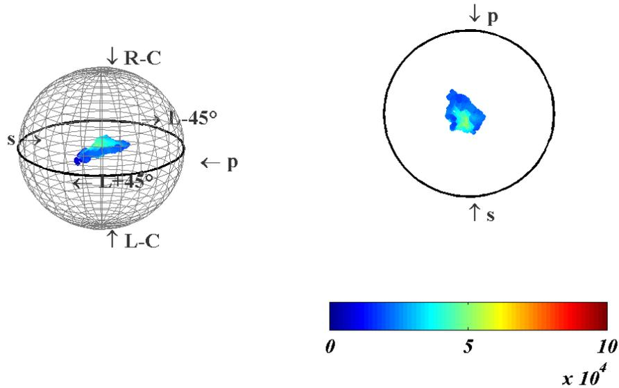
Fig. 19. Polarization states for the bulk black sample- unpolarized illumination.
