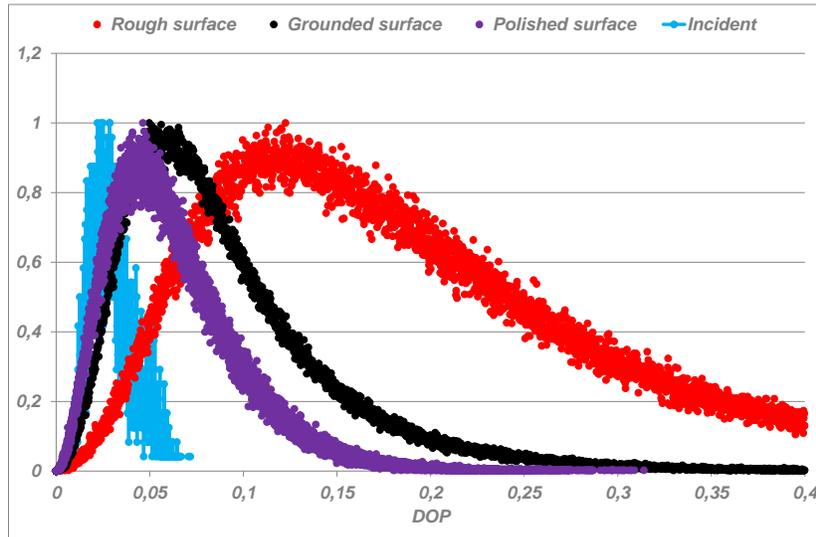
Fig. 6. Normalized dop histograms measured for the lambertian, grounded and polished surfaces- Unpolarized illumination.
