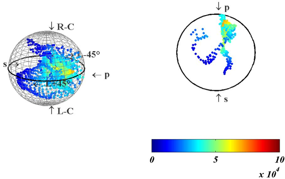
Fig. 17. Polarization states for the bulk white sample- unpolarized illumination.
