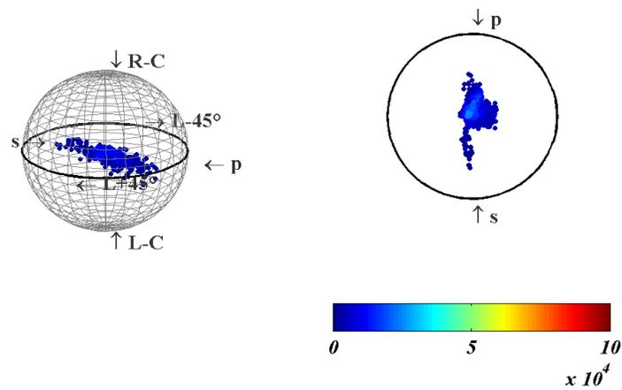
Fig. 8. Polarization states on the Poincaré sphere for the grounded surface sample (S<sub>2</sub>). Unpolarized illumination.
