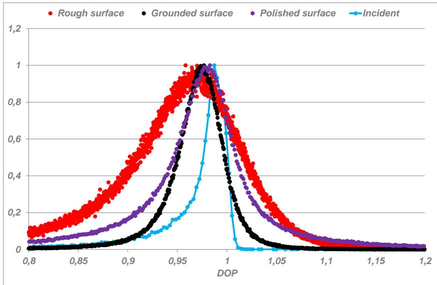
Fig. 3. Normalized dop histograms measured for the lambertian (in red), grounded (black) and polished (in purple) surfaces- Case of polarized illumination.
