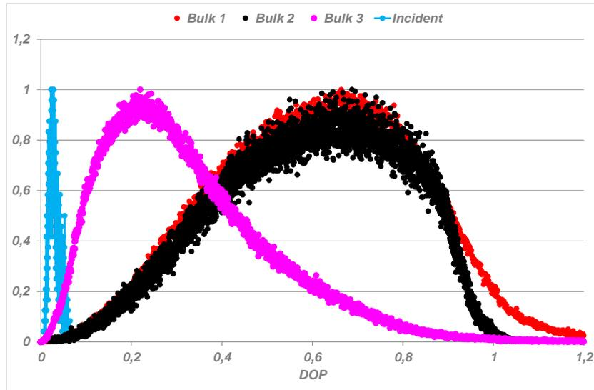
Fig. 16. Normalized dop histograms of the 3 bulk samples –Unpolarized illumination B<sub>1</sub>: white bulk, B<sub>2</sub>: grey bulk, B<sub>3</sub>: black bulk.
