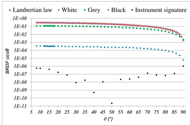
Fig. 11. ARS curves of the 3 bulk samples.
