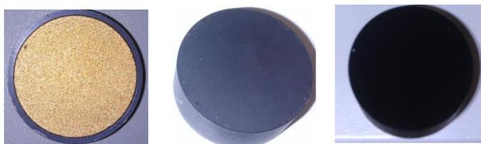
Fig. 1. Photographs of the 3 surface samples: lambertian (left), grounded (middle) and polished (right).
