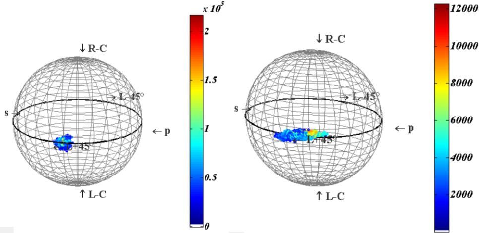
Fig. 5. Polarization states on the Poincaré sphere for the grounded (left,  $S_2$ ) and the polished (right,  $S_3$ ) black surfaces - Polarized illumination.
