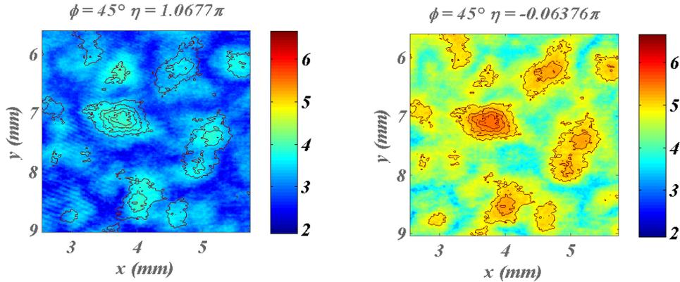
Fig. 10. Minimum ( $\eta = \pi$ - left figure) and maximum ( $\eta = 0$ - right figure) intensity of the scattering pattern at the system output, with the grey levels in logarithmic scale. Data are normalized to the integration time. The area of investigation is  $3\text{mm} \times 3.5\text{mm}$ .
