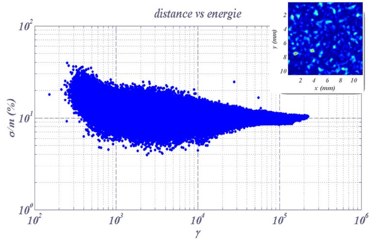
Fig. 16. Distance function of the scattering pattern versus the grey levels. The region of investigation is given at the right, top. The distance provides a criteria for the quality of the LMS procedure (see text related to Fig. 8).
