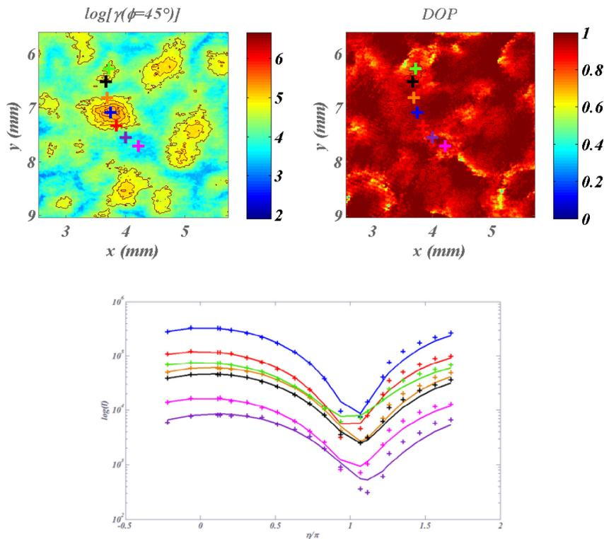
Fig. 13. complete polarization curves (bottom figures) measured for the pixels identified in the top figure across the frontiers of a grain size.
