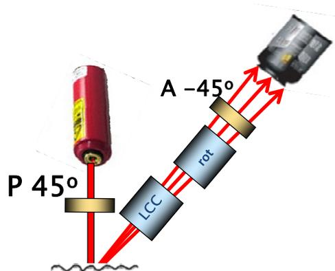
Fig. 9. Basic polarization set-up for analysis of the scattering pattern.
