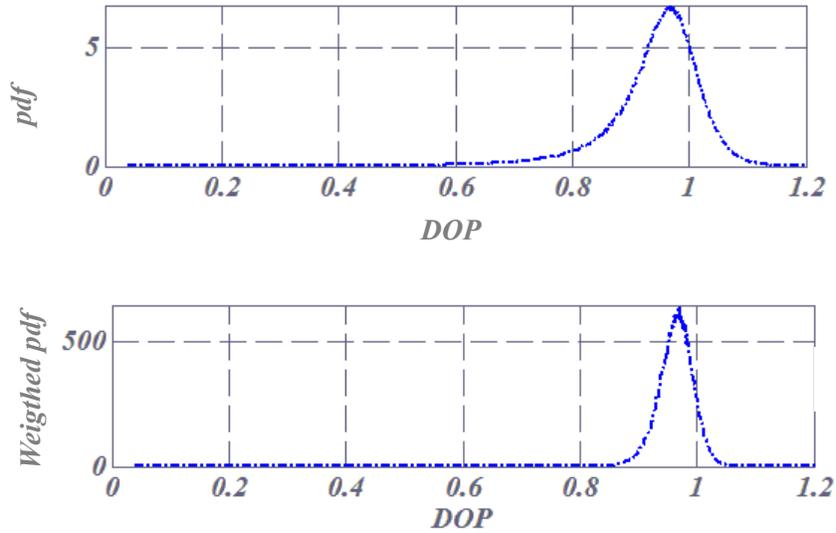
Fig. 15. dop histograms of the scattering pattern, *weighted (bottom) or not (top) by the energy levels.*
