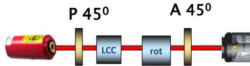
Fig. 1. Basic polarization set-up for specular optics.
