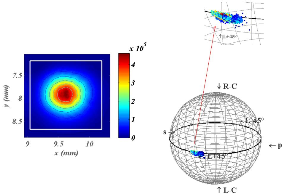
Fig. 6. Polarization states on the Poincaré sphere (right figure- with a zoom on the top), plotted for the square region of the left figure.
