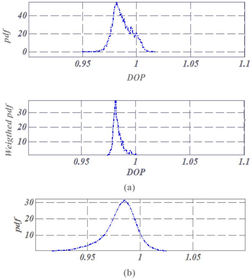
Fig. 7. a: dop histograms measured within the investigation area, weighted (middle figure) or not (top figure) by grey levels (see text). b: calculation of a dop histogram ((see text)) of full polarized pattern in the presence of Gaussian noise with 10% root mean square.
