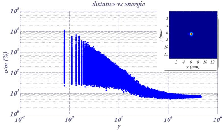
Fig. 8. Histogram of the distance function versus the grey levels. The region of investigation is given at the right, top. The distance provides a criteria for the quality of the LMS procedure (see text).
