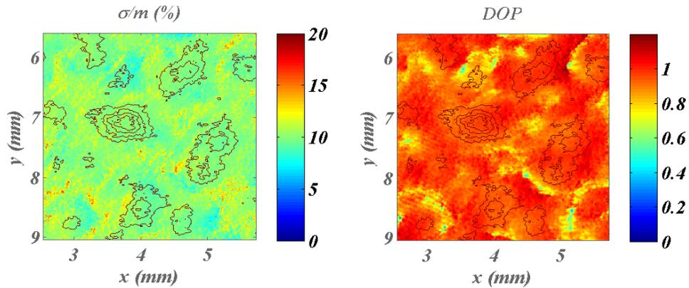
Fig. 12. mapping the dop (right figure) of the surface scattering pattern and its associated distance (left figure).
