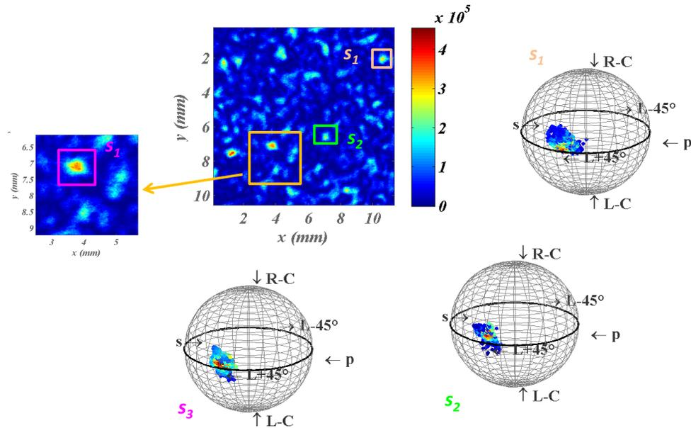
Fig. 14. Polarization states on the Poincaré sphere for different areas within the speckle pattern.
