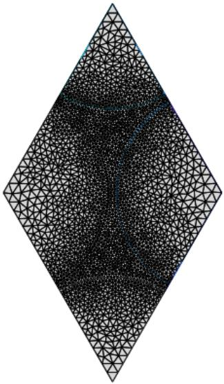
Meshing of a basic rhombic cell with 4628 triangles.
