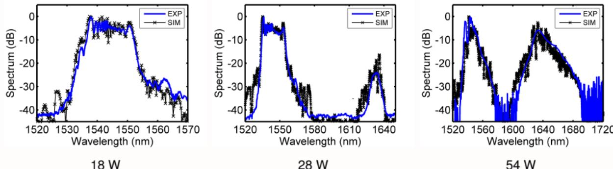
**Figure:** Output spectra recorded from 1.8m long 2.6  $\mu\text{m}$  core As<sub>2</sub>S<sub>3</sub> MOF for 3 input powers
