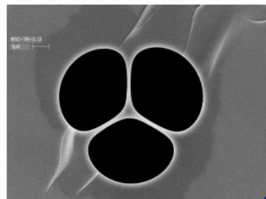
suspended core MOF made of As<sub>2</sub>S<sub>3</sub>, core size ≈ 2.3 μm (ICB, Université de Bourgogne)
