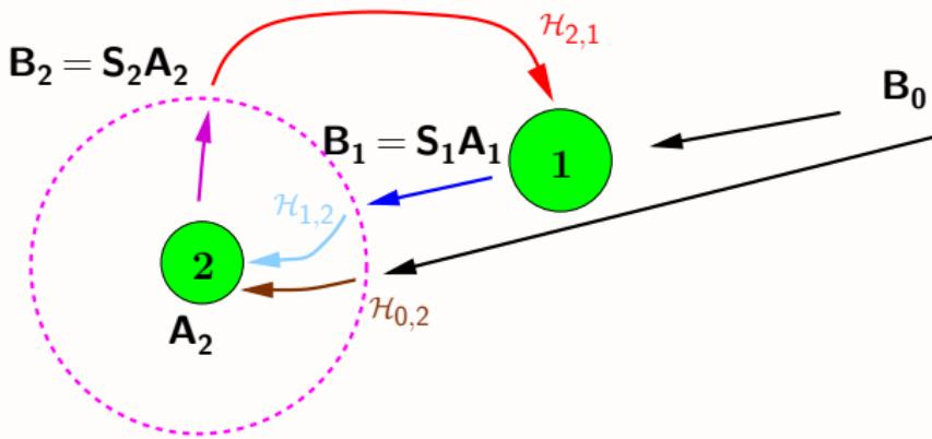
**Figure:** Scheme of principle of the multipole method: self-consistency of the incident and scattered fields by the set of inclusions
