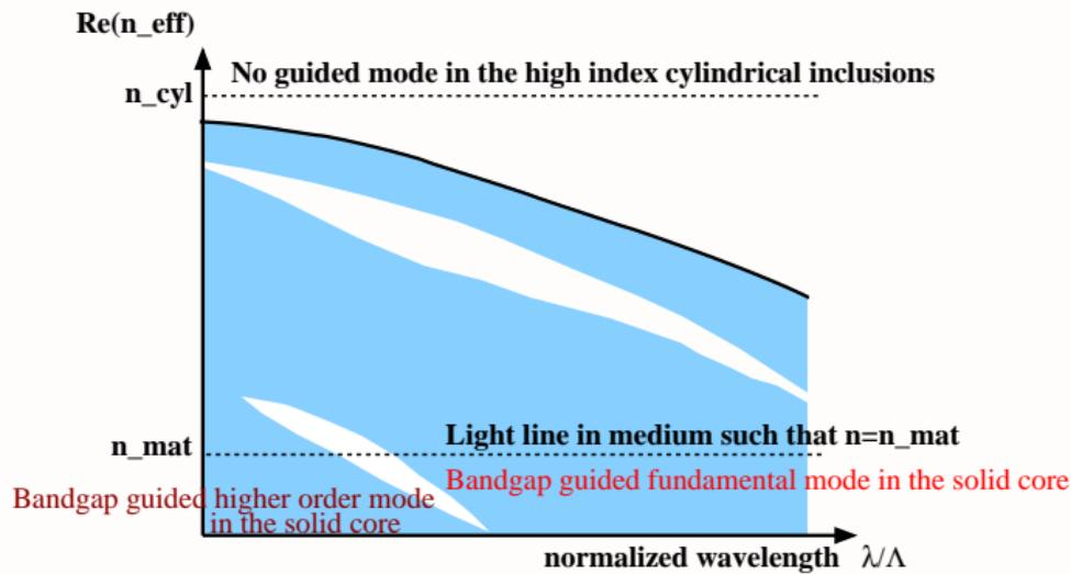
**Figure:** Schematic band diagram of a periodic array of inclusions of high refractive index  $n_{\text{cyl}}$  in a low refractive index matrix  $n_{\text{mat}}$  such that  $n_{\text{cyl}} > n_{\text{mat}}$  together with the dispersion curves of the fundamental mode and a higher order mode of the finite size MOF such that  $n_{\text{core}} = n_{\text{mat}}$ .
