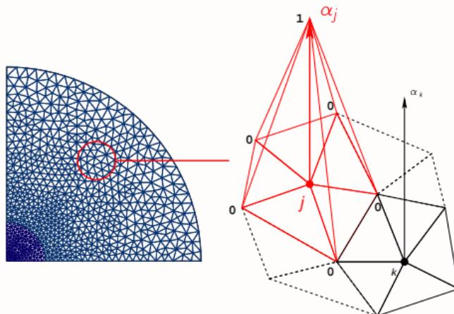
**Figure:** Mesh on a quarter of the fiber cross section and form functions in the scalar case
