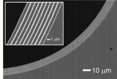
Bragg fiber made of polymer and chalcogenide (MIT/Harvard University)
