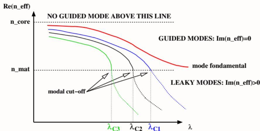
Figure: Scheme of the dispersion curves  $\text{Re}(n_{\text{eff}})$  of the first modes
