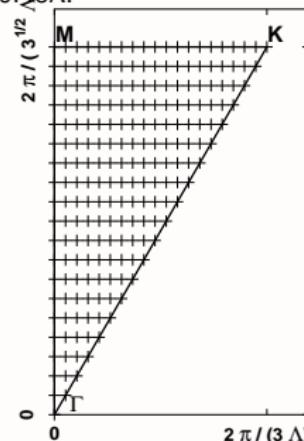
Example of sampling points in the irreducible part of the Brillouin zone (IBZ) for a triangular lattice. 210 points are used in this case to sample in 2D the IBZ.
