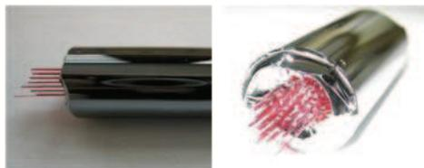
Fig. 1.  $\text{As}_2\text{S}_3/\text{As}_{38}\text{Se}_{62}$  preform:  $\text{As}_2\text{S}_3$  sticks are thread in the  $\text{As}_{38}\text{Se}_{62}$  holey preform.
