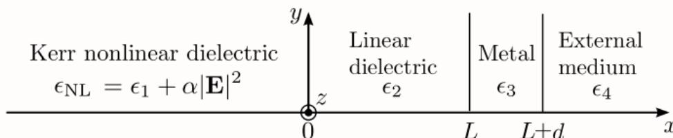
Geometry of the 4-layer nonlinear model used to study 3-layer structures.
