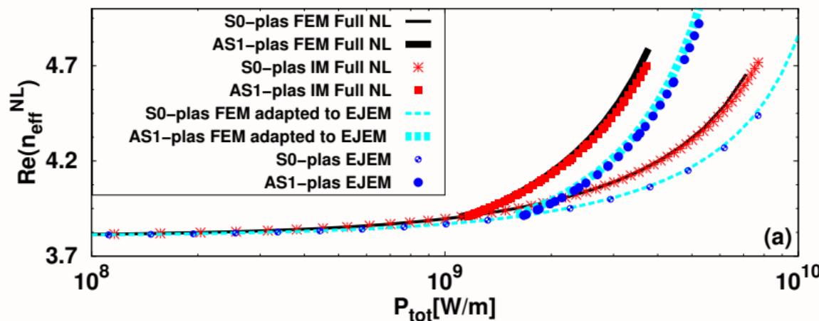
**Isotropic case:** nonlinear dispersion relation for the symmetric and asymmetric modes as a function of total power  $P_{tot}$ .  $\lambda = 1.55 \mu\text{m}$ ,  $d_{core} = 400 \text{ nm}$ , and  $n_2 = 2.10^{-17} \text{ m}^2/\text{W}$ , and for  $\epsilon_{\perp} = 0.042$ ,  $\epsilon_{//} = 9.07$ .
