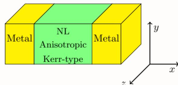
Full slot with its metamaterial nonlinear core
