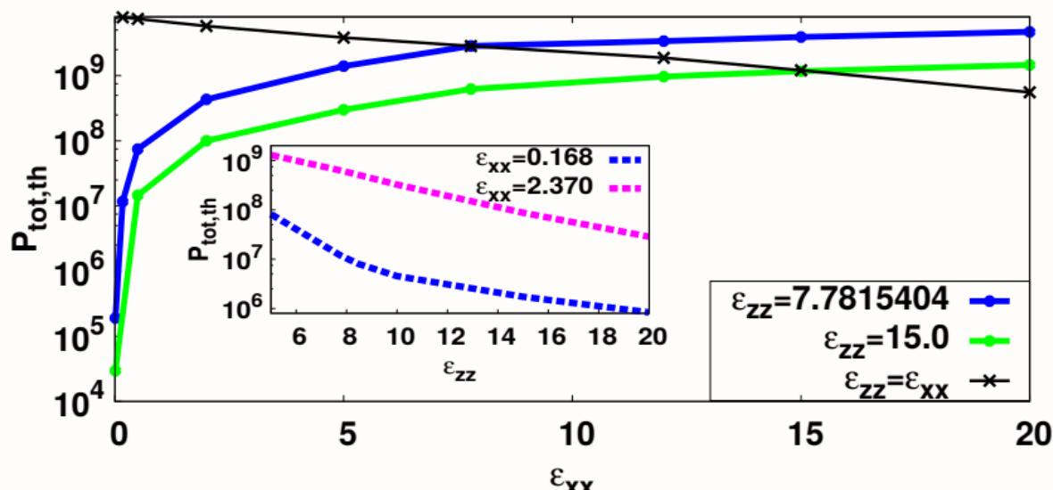
**Anisotropic case:** Power threshold  $P_{tot,th}$  as a function of linear transverse permittivity  $\epsilon_{xx}$  in the elliptical case for two longitudinal permittivity  $\epsilon_{zz}$  values. Isotropic case is shown by the black curve. Inset:  $P_{tot,th}$  as a function of  $\epsilon_{zz}$  for two  $\epsilon_{xx}$  values.
