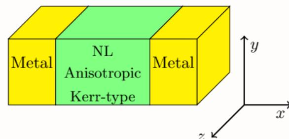
Full slot with its metamaterial nonlinear core
