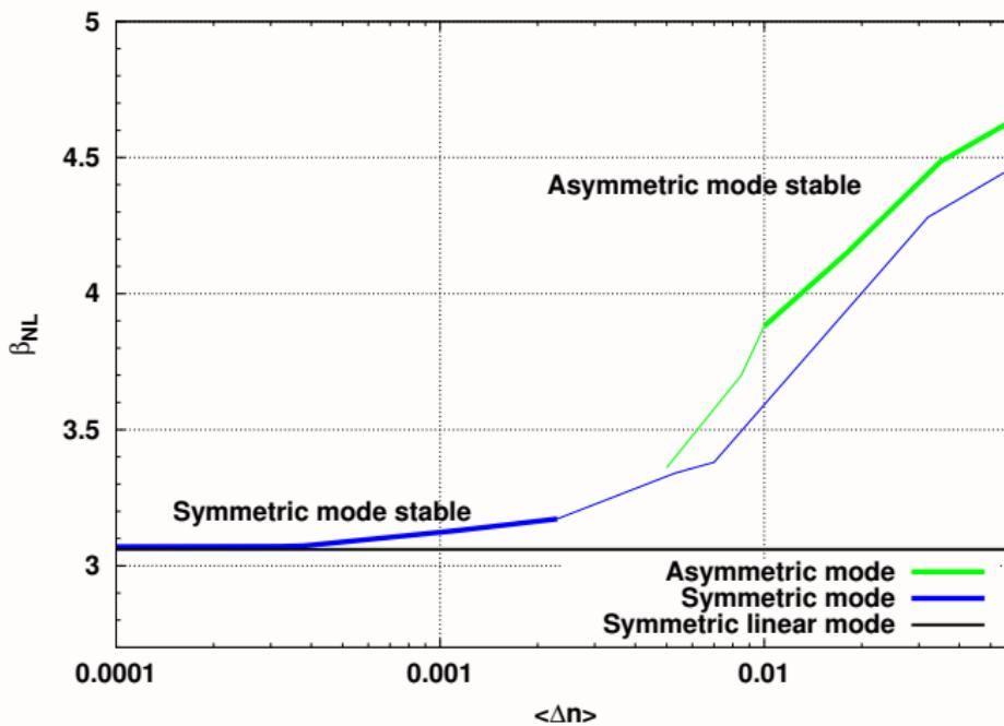
Dispersion curves with stability results for the symmetric and asymmetric modes from FDTD simulations,  $d = 500$  nm amorphous Si core surrounded by gold
