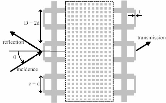
Fig. 3. Schematic representation of the in-coupling gratings having twice the period  $D = 2d$  and thickness  $t$ , made of the same dielectric material as the crystal. Incident wave comes from the left and generates a reflected and a transmitted waves
