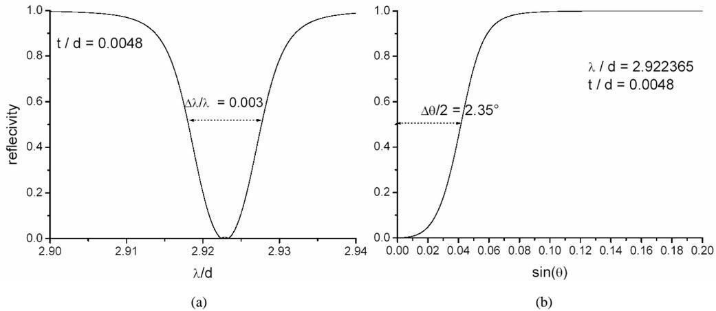
Fig. 6. As in Fig. 5 but with thicker supplementary gratings,  $t/d = 0.0048$  instead of 0.002
