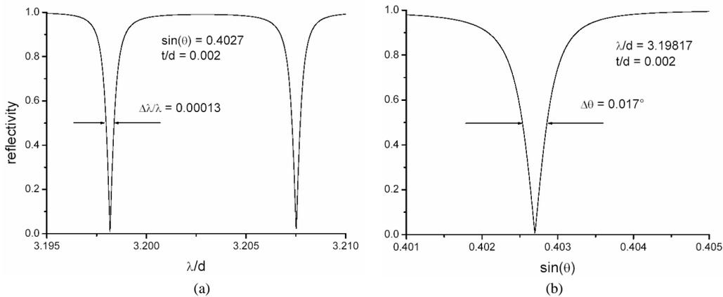
Fig. 4. Resonances in the spectral (a) and angular (b) responses of the system presented in Fig. 3 with  $t/d = 0.002$  and working in non-normal incidence. The wavelength and angular parameters are indicated in the figure.
