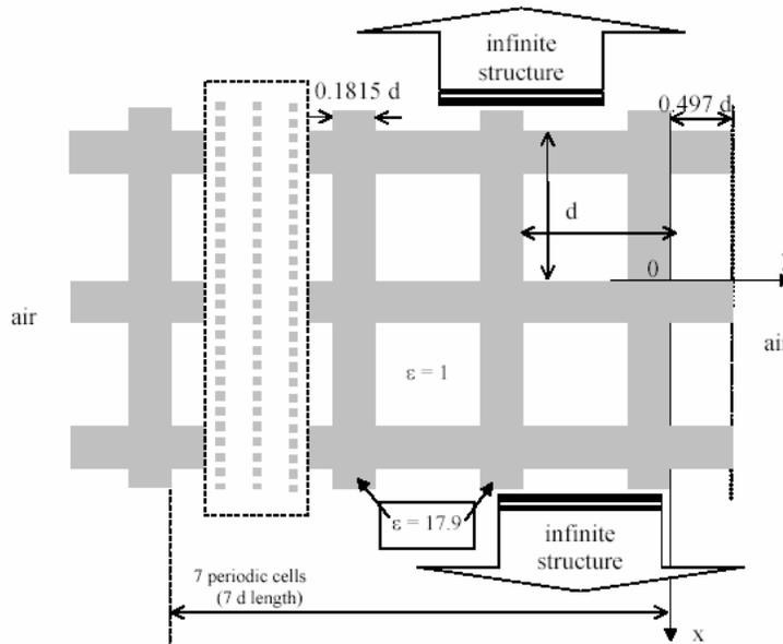
Fig. 1. Schematic representation of a two-dimensional photonic crystal slab and its optogeometrical parameters
