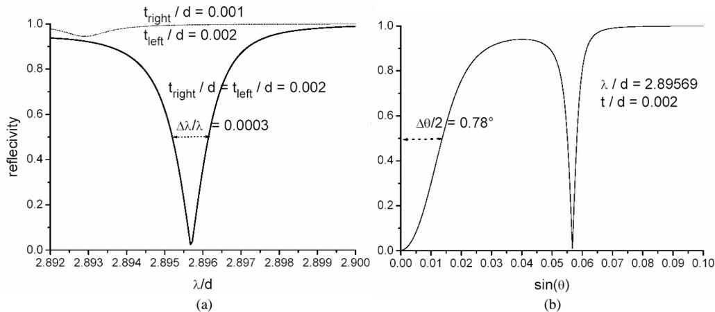
Fig. 5. As in Fig. 4 but working close to normal incidence. The thin curve in Fig. 5(a) corresponds to different thicknesses of the supplementary gratings in Fig. 3, the left grating is  $0.002d$  thick, while the right grating is twice thinner.
