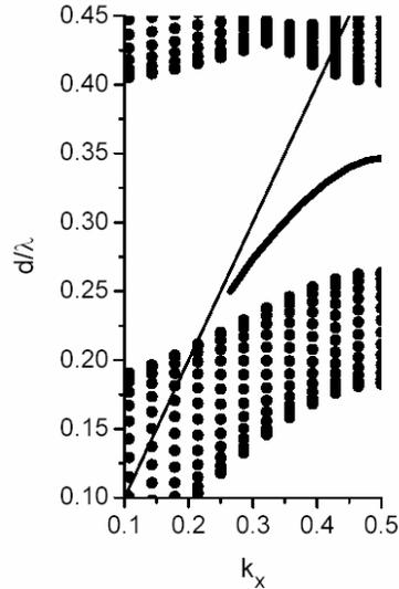
Fig. 2. The band-gap structure of the photonic crystal presented in Fig. 1 and the dispersion curve of the guided surface-induced TM mode. The parameter  $k_x$  is the normalized x-component of the wavevector  $\vec{k}$ :  $k_x = \frac{2\pi}{d} \vec{k} \cdot \vec{x} = \frac{\lambda}{d} \sin \theta$  (for  $\theta$ , see Fig. 3). The thin line presents the light cone and the thick line, the mode dispersion curve
