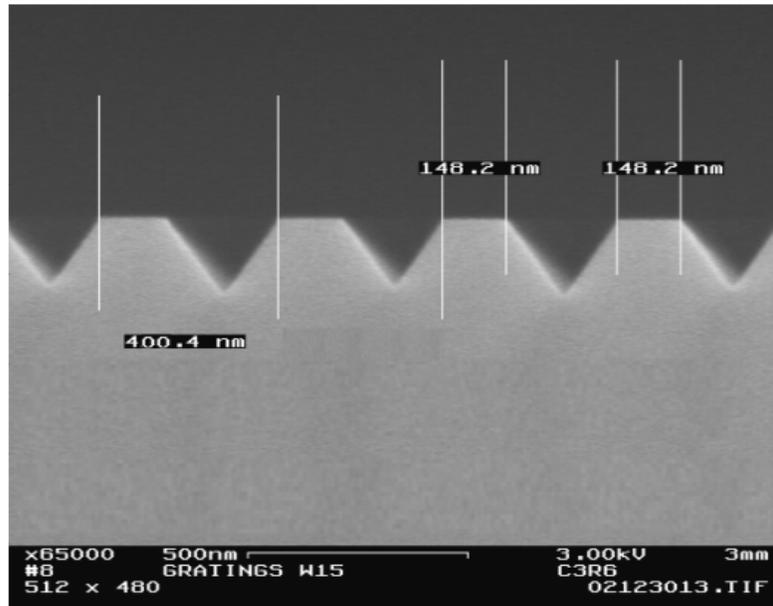
Fig. 3 SEM picture of a Si grating with triangular profile and flat top region.
