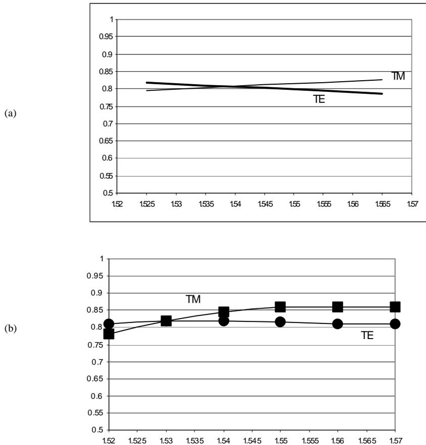
Fig. 4. Theoretical (a) and experimental (b) efficiency of a Si grating covered with Au layer and measured from the wafer side. Period  $0.4 \mu\text{m}$ , flat region  $148 \text{ nm}$ , angle of incidence inside the wafer  $33.7^\circ$ .
