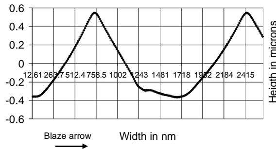
Fig. 1. Measured profile of the echelette grating (master no. 1117 ruled by Richardson Grating Laboratory, Spectronic Instruments, Inc., Thermo Optek Co.).
