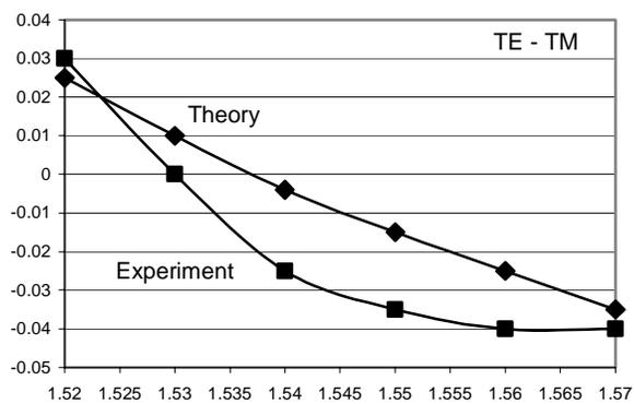
Fig. 5. Spectral variation of the polarization difference (TE minus TM efficiency).
