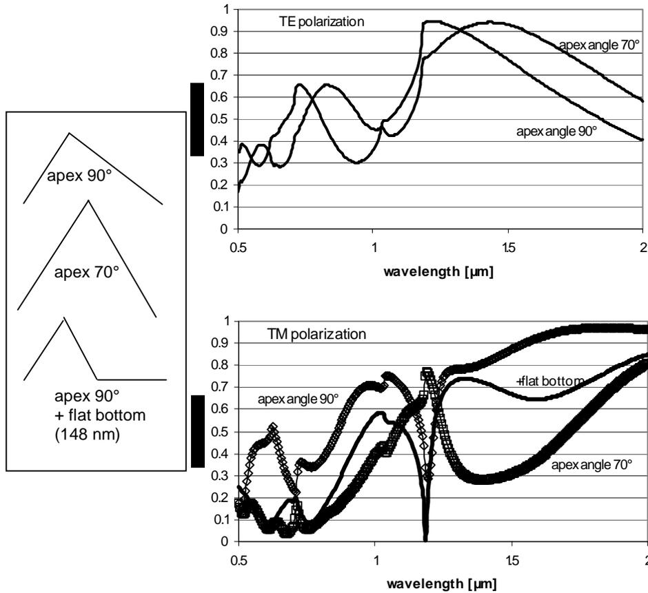
Fig. 2. Diffraction efficiency of three different echelette gratings with profiles presented in the inset. 600 gr/mm, measurements at  $8^\circ$  angular deviation (A.D.) (a) TE polarization, (b) TM polarization.
