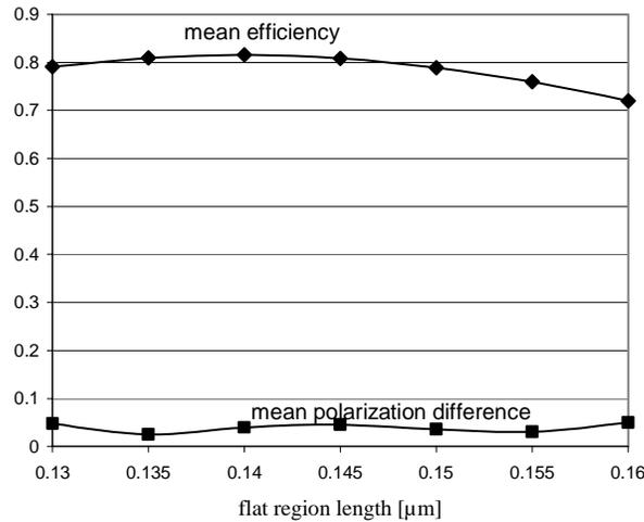
Fig. 6. Mean efficiency and mean polarization difference within the spectral region 1.52-1.57  $\mu\text{m}$  as a function of the flat region width of the profile.
