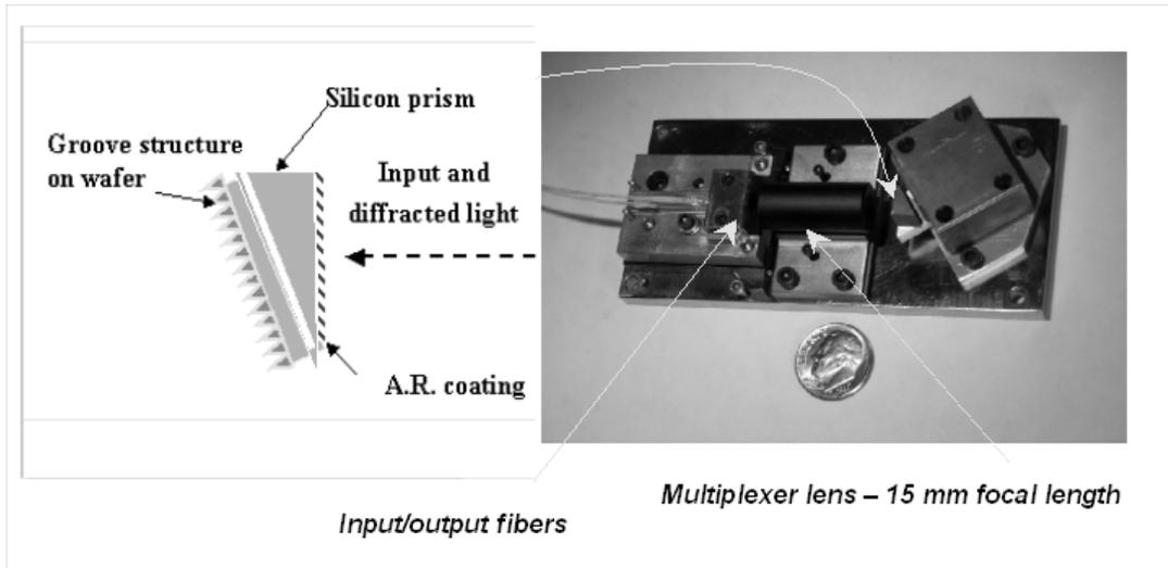
Fig. 7. Schematic representation and general view of the device.
