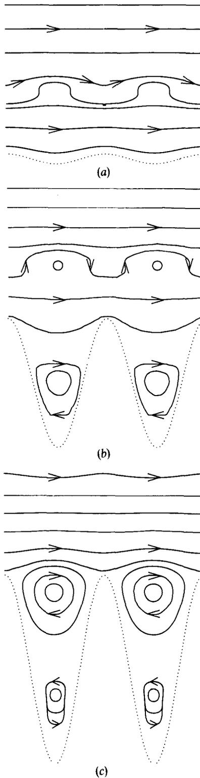
Figure 6. Energy flow distribution above the surface of the grating described in figure 5. In (a)  $h/d=0.10$ ; in (b)  $h/d=1.30$ ; in (c)  $h/d=1.93$ .
