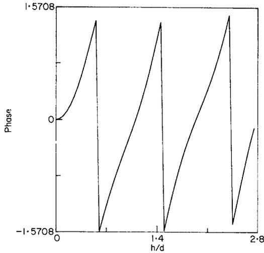
Figure 5. Phase of the 0th reflected order against groove depth to period ratio for a perfectly conducting grating of period  $d=0.3\ \mu\text{m}$  at wavelength  $0.6328\ \mu\text{m}$ : sinusoidal profile. Angle of incidence  $\theta = \arcsin(0.6328)$ .
