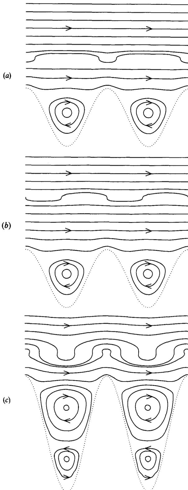
Figure 4. Same as for figure 2, but for very deep gratings. Figure 4(b) is not in the Littrow mounting ( $\sin \theta = 0.6328$ ), but at  $\theta = \arcsin(0.85)$ . In (a)  $h/d = 0.72$ ; in (b)  $h/d = 0.72$ ; in (c)  $h/d = 1.44$ .
