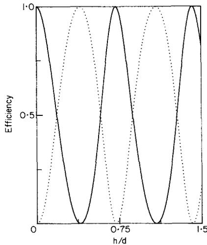
Figure 1. Diffraction efficiency of the 0th (solid line) and the  $-1$ st (dotted line) reflected order against groove depth to period ratio in the Littrow mounting for a perfectly conducting grating of period  $d=0.5\ \mu\text{m}$  at wavelength  $0.6328\ \mu\text{m}$ : sinusoidal profile.
