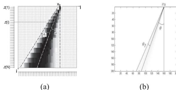
Fig. 1. (a) linear antenna model in an image containing a fuzzy contour; (b) hand-made fuzzy triangle contour characterized by the main orientations  $\theta$  and offsets  $x_0$  in the image
