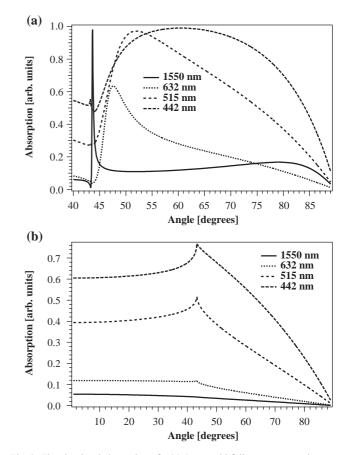
Fig. 2. The simulated absorption of a 29.5-nm gold foil on a quartz substrate at the photon energies considered in this work. The film thickness was optimized for the infrared line. (a) displays the p-polarization spectra, while (b) shows the corresponding s-polarization.
