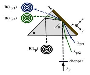
Fig. 1. Schematics of the experimental arrangement for SPAC. The gold film is defined by the *xy*-plane. The incident infrared beam is labeled  $\lambda_p$ , while all the incident visible beams are labeled  $\lambda_{pri}$ ; with *i*=1, 2, ..., and the corresponding reflected beams are labeled by *R*.
