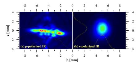
Fig. 3. The influence of the polarization state of the IR pump beam on the reflected probe beam profile. In (a), the diffracted reflected probe beam  $R(\lambda_{prl})$  is recorded under the influence of the IR SP, while in (b) no effect can be observed due to s-polarization state of the IR beam.
