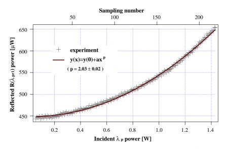
Fig. 5. The measured variation of SPAC magnitude. Reflected visible power as a function of incident infrared excitation  $\lambda_p$  power. A 20-mW p-polarized  $\lambda_{pr1}$  beam incident at 60° undergoes resonant absorption in the film to generate the reflected power  $R(\lambda_{pr1})$ . As can be seen from the inset, a quadratic fit describes the magnitude of the SPAC fairly well.
