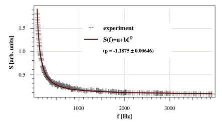
Fig. 6. The measured frequency dependence of SPAC. The modulation of the reflected visible  $R(\lambda_{prl})$  power as a function of the modulated infrared excitation  $\lambda_p$  power (symbols). The solid curve represents a numeric fit to an inverse function which appears to describe the frequency dependence of SPAC well.
