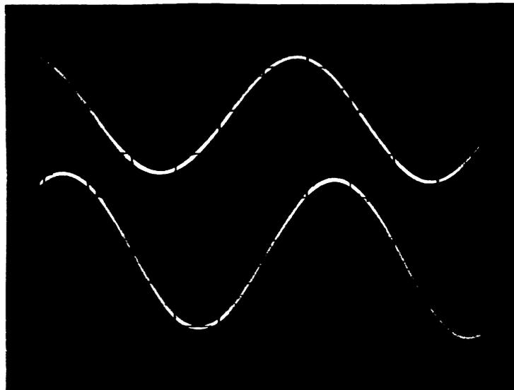
Figure 2-Parallely coherence demultiplexed signals generated by two polarization couplers along a single fibre (scales are the same for both signals: 100 mV per division)
