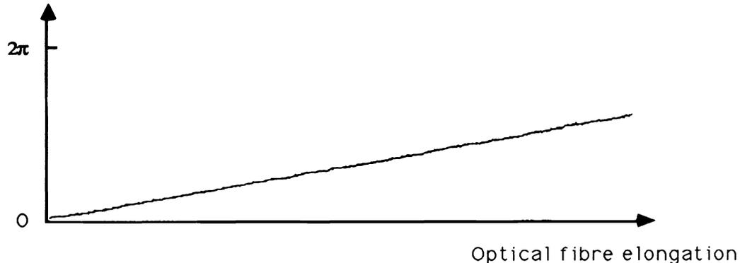
Figure 3-Phase variation between the two signals when the optical fibre is elongated between the polarization couplers.
