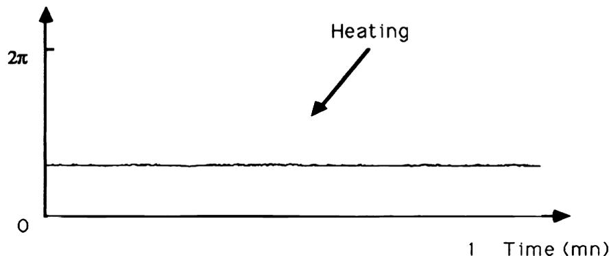
Figure 4-Phase measurement between the two signals when heating is produced outside the region comprized between the polarization couplers
