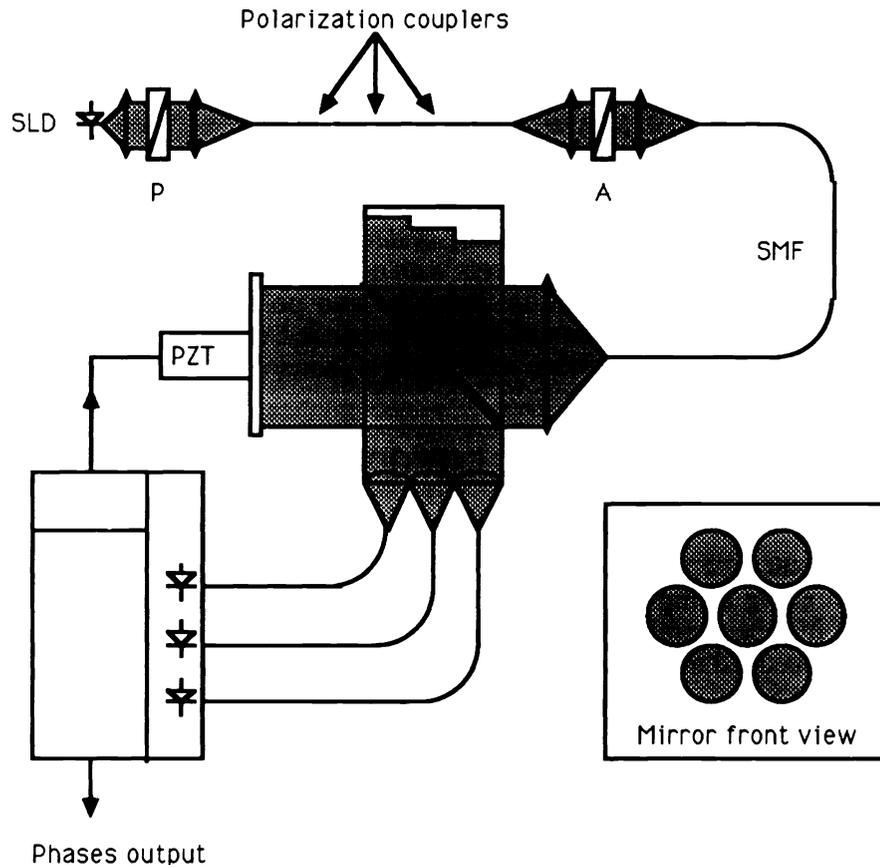
Figure 1-Scheme of the white-light polarimetric quasi-distributed system with parallel receiver
