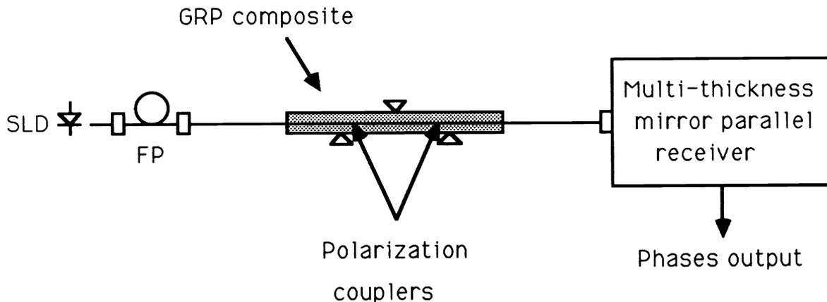
Figure 5- All fibre configuration for composite testing
