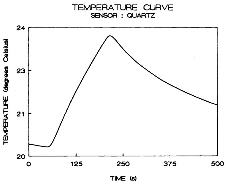
Fig. 7. Response of a Prototype Temperature Sensor
