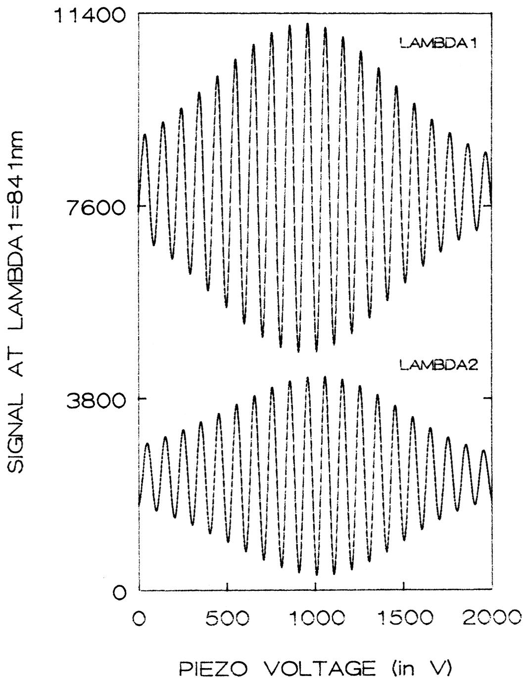
Fig. 4. Experimental Phase Signals for both LED
