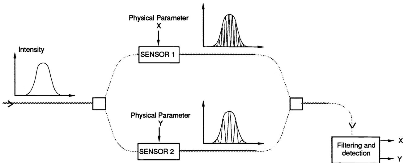
Fig.1. Schematic description of the spectral modulation encoding techniques
