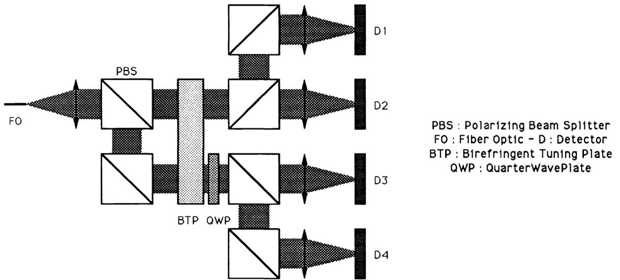
Fig. 2. Functional description of the optical detection head
