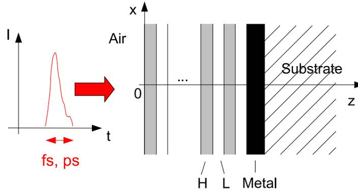
Fig. 1. Schematic and coordinates of the system under study. H: high refractive index layer, L: Low refractive index layer
