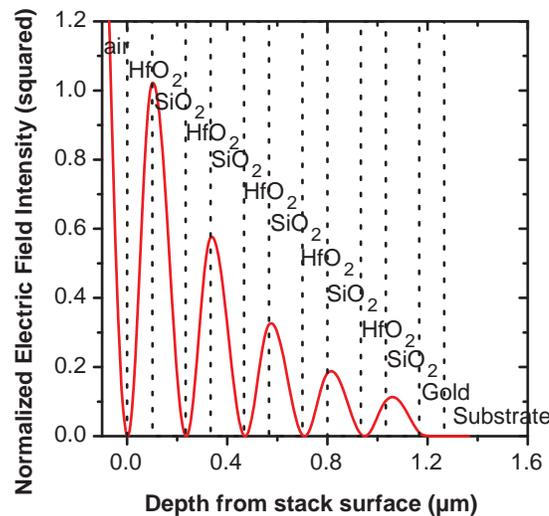
Fig. 8. Electric field distribution in the stack *Silica/Gold/(SiO<sub>2</sub>/HfO<sub>2</sub>)<sup>5</sup>*, calculated at 800nm.
