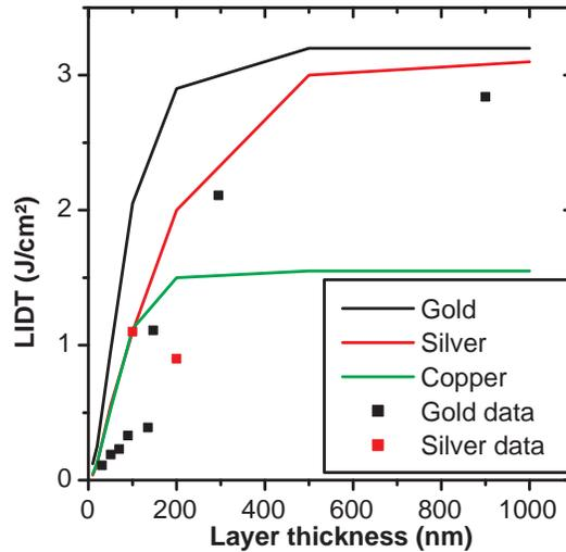
Fig. 6. Theoretical thresholds for single layer metal film with different thicknesses, calculated at 800nm, 50fs, using the material parameters listed in table 2. The experimental data correspond to the values given in table 1.
