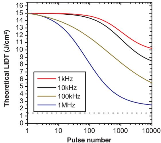
Fig. 10. Calculation of the fluence needed to reach the melting point of the gold film in the case of a MMLD mirror (*Silica/Gold/(SiO<sub>2</sub>/HfO<sub>2</sub>)<sup>5</sup>*) irradiated with different number of laser pulses at various repetition rates. The dotted line corresponds to the fluence needed to initiate damage in the high index material of the stack.
