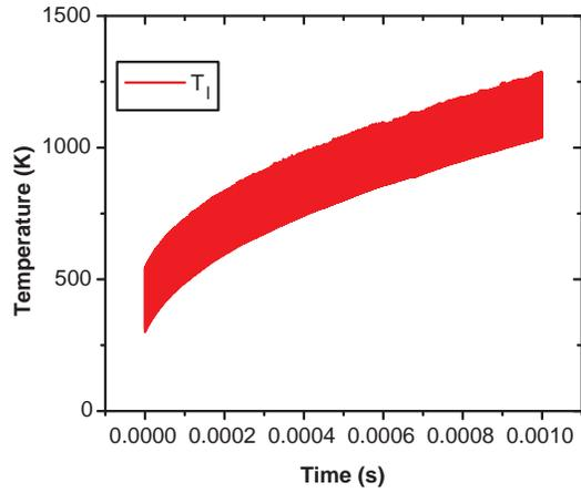
Fig. 4. Temperature evolution as a function of time of a metal/multidielectric stack (same design as in Fig. 3) submitted to multiple pulses irradiation. The temperature is plotted in the metal film, where it reaches its maximum value. The irradiation conditions are: pulse duration of 500fs, 1MHz repetition rate,  $3.5J/cm^2$  per pulse, and 800nm wavelength.
