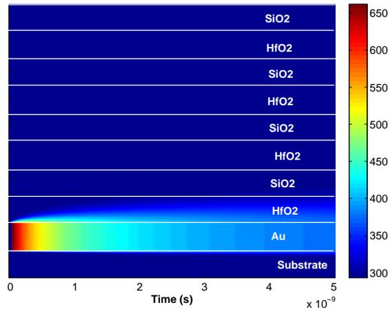
Fig. 3. Calculations of the lattice temperature with the two temperatures in the case of a metal multidielctric mirror composed of a dielectric mirror  $((HfO_2/SiO_2)^4)$  on a gold film, deposited on a silica substrate. The laser irradiation is  $4J/cm^2$  with a pulse duration of 500fs at 800nm. The temperature in the stack is plotted as a function of time up to 5ns after the end of the pulse in order to observe the temperature decay and diffusion.
