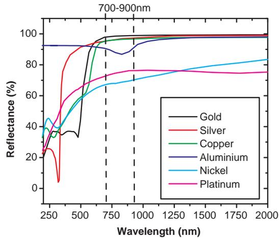
Fig. 5. Reflectance of commonly used metals as a function of wavelength from 200 to 2000nm. The plot is extracted from the data in [15]
