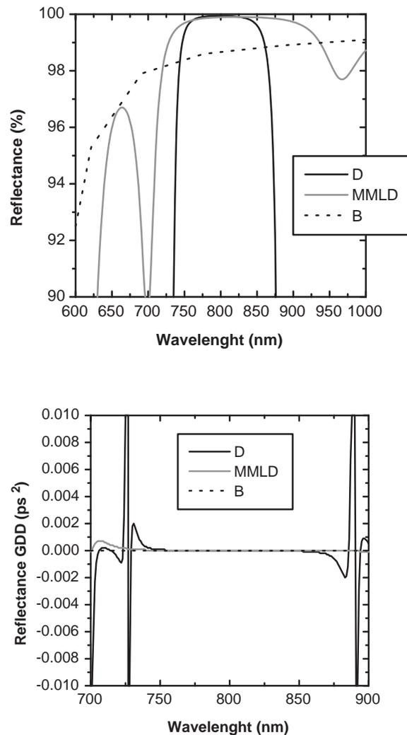
Fig. 7. A comparison of the Reflectance and Group Delay Dispersion of a dielectric mirror  $\text{Silica}/(\text{HfO}_2/\text{SiO}_2)^{15}/\text{HfO}_2$  (D), a MMLD mirror  $\text{Silica}/\text{Gold}/(\text{SiO}_2/\text{HfO}_2)^5$  (M), and a metallic gold mirror (B).
