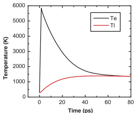
Fig. 2. Calculated temperature profiles ( $T_e$ : electronic temperature,  $T_l$ : lattice temperature) at the surface of a gold film irradiated by a pulsed laser. Laser wavelength is 800nm, pulse duration is 500fs and the fluence is  $0.85J/cm^2$ . The gold film thickness is 100nm, and the substrate is silica.
