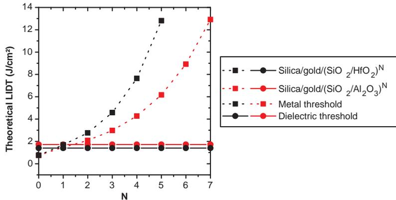
Fig. 9. Case of MMLD mirrors with different high index materials: calculation of the fluence needed to reach the melting point of the gold film (dotted lines) and comparison to the fluence needed to initiate damage in the high index material (plain line).
