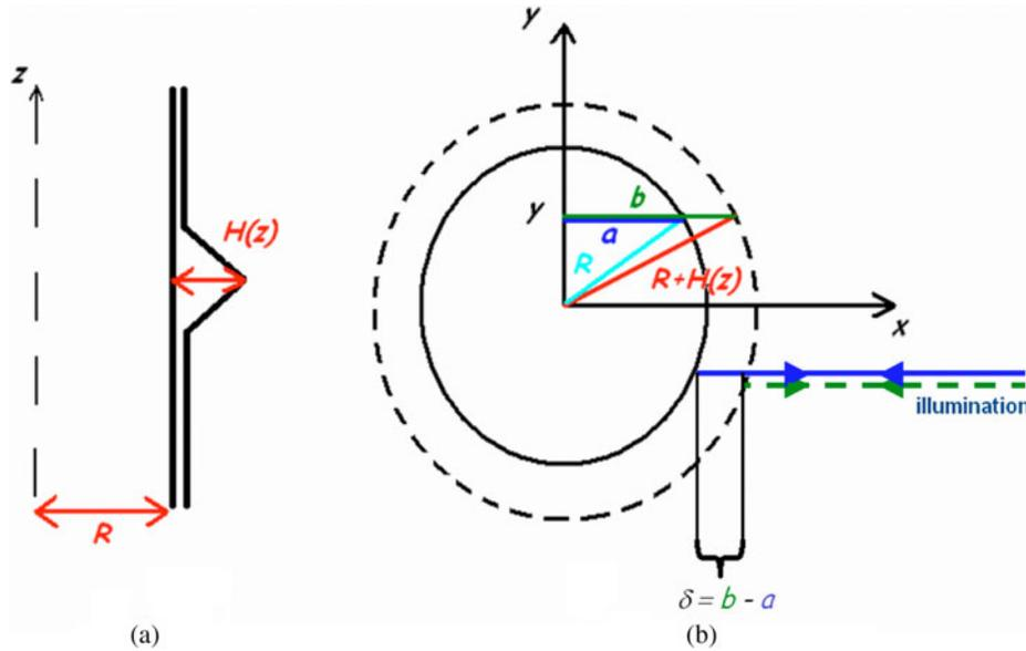
Fig. 10. (a) Fringe calculations in the case of circumferential deformation in the  $(x, z)$  plane and (b) geometrical parameters for fringe calculation in the  $(x, y)$  plane.
