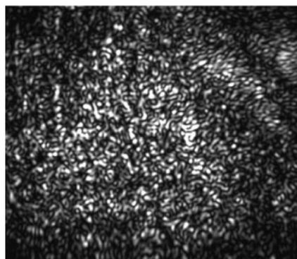
Fig. 3. Speckle pattern observed when metal fuel cladding is illuminated with a He-Ne laser.
