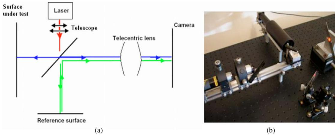
Fig. 6. (a) Out-of-plane configuration with flat-surface sample and (b) real setup.
