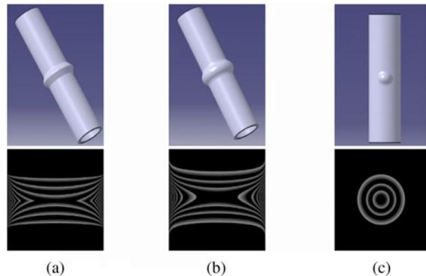
Fig. 11. Views of different calculated deformation and fringes: (a) triangular, (b) Gaussian, and (c) bulge.
