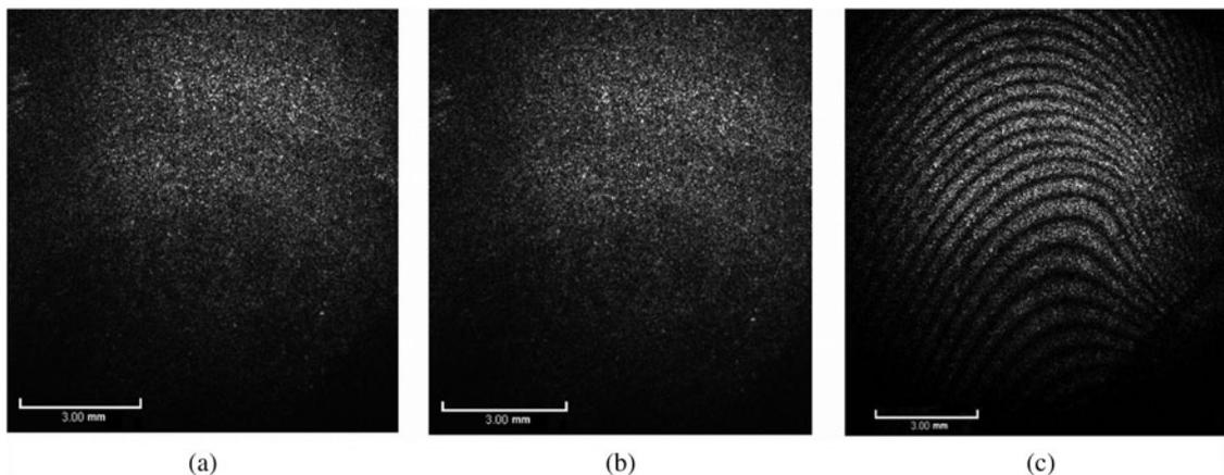
Fig. 5. (a) Speckle pattern before deformation, (b) speckle pattern after deformation, (c) fringes obtained by subtraction of the two previous pictures (b)-(a).
