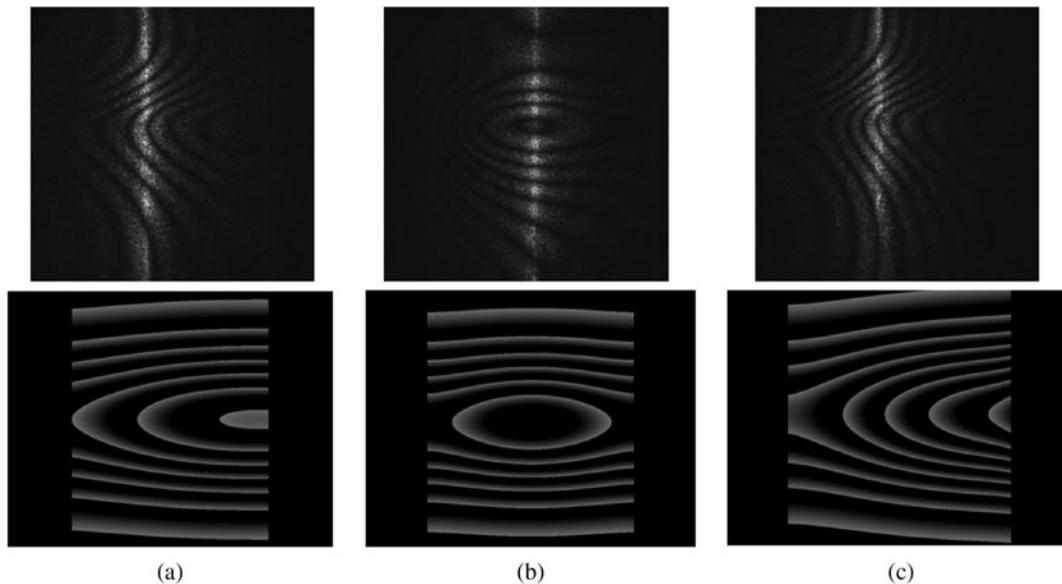
Fig. 13. Comparison between experimental results and calculation for different rotation angles: (a) 20 deg, (b) 90 deg, and (c) 180 deg.
