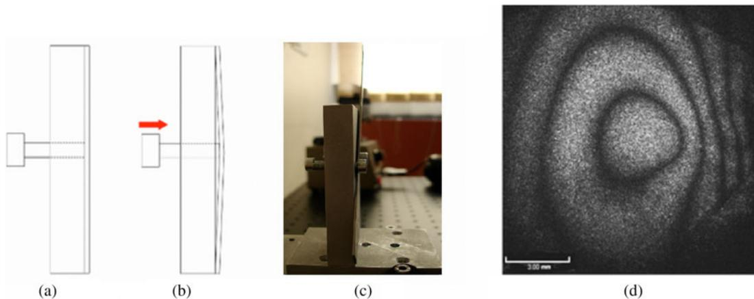
Fig. 7. (a) Flat surface in the initial state, (b) constraint is applied from the backside of the flat surface, (c) picture of the real sample, and (d) example of fringes obtained with this sample.
