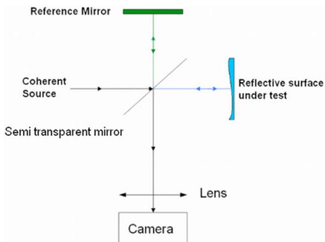
Fig. 1. Experimental configuration of an interferometer to measure the topography of a reflective surface.
