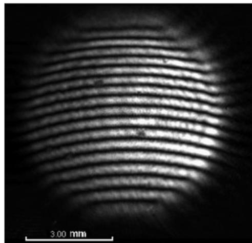
Fig. 2. Example of an interference pattern obtained with Michelson interferometer.
