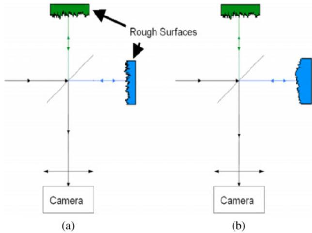
Fig. 4. Speckle interferometry (a) before deformation and (b) after deformation.
