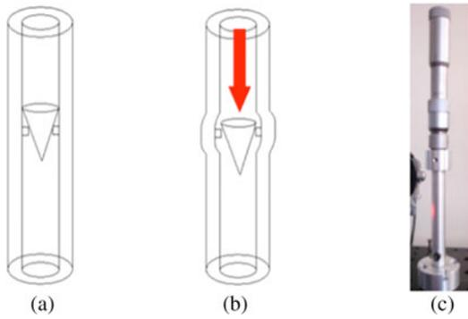
Fig. 8. (a) Cylinder in the initial state, (b) constraints are applied from the inside of the pipe by pressure on a cone, and (c) picture of the real sample.
