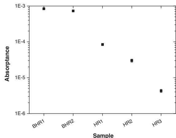
**Fig. 10.** Measured absorptance on the different laser mirrors.
