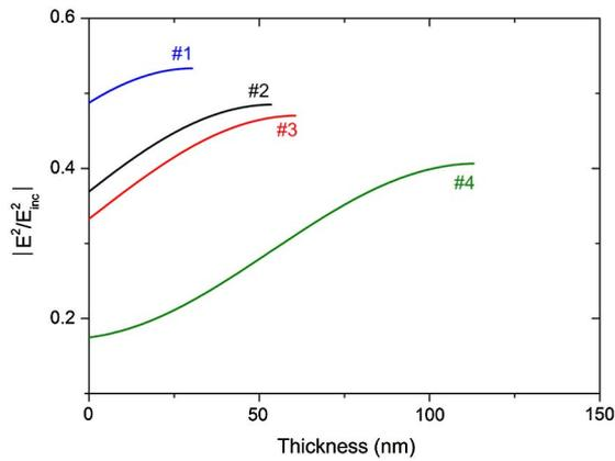
**Fig. 8.** Normalized electric field distributions in the  $\text{Nb}_2\text{O}_5$  films of different thicknesses, plotted for 1060 nm wavelength.
