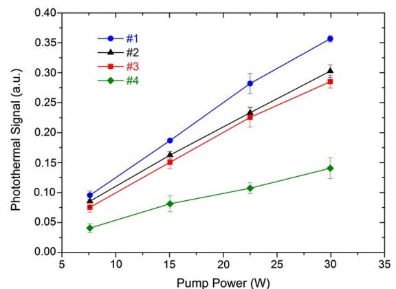
Fig. 7. Evolution of the photothermal signal achieved by LIT method with the increased heating laser power (pump power).
