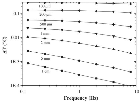
**Fig. 2.** Temperature modulation in the case of periodic surface heating of a silica sample, with different frequencies. Results are plotted for different beam diameters with 100 μW absorbed power.
