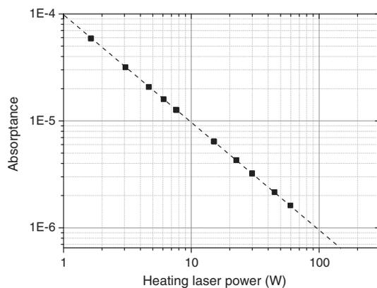
Fig. 6. Noise-equivalent absorbance with the heating laser power.
