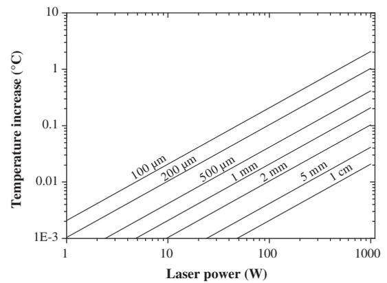
**Fig. 1.** Steady-state temperature increase obtained from Eq. (1) as a function of laser power for different beam diameters.  $A = 1e-6$ ,  $K = 1.36 \text{ W/m/K}$ .
