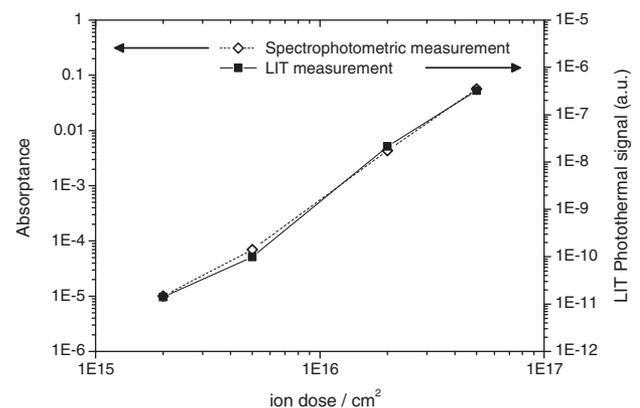
**Fig. 5.** Absorptance of the calibrate sample measured by classical spectrophotometric method and the photothermal signal measured by LIT method (normalized by the incident intensity), depending on the ion dose.
