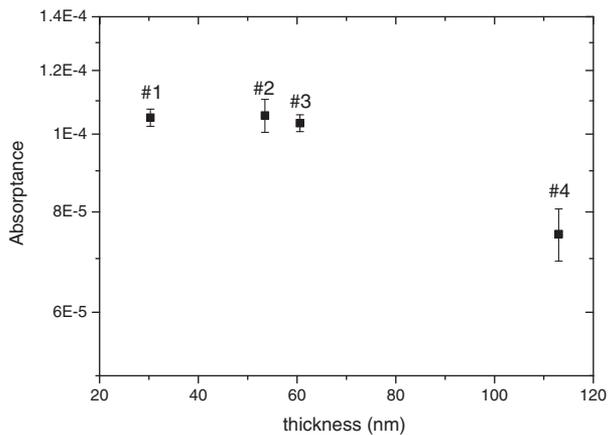
**Fig. 9.** Calculated absorptance for the  $\text{Nb}_2\text{O}_5$  coatings with different thicknesses.
