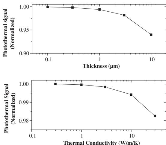
**Fig. 4.** Evolution of the photothermal signal in the case of a film on a fused silica substrate as a function of (a) thickness of the film and (b) thermal conductivity of the film. The simulations have been done for a frequency of 0.25 Hz and the beam size of 200  $\mu\text{m}$ , as in the experiment.
