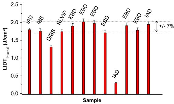
Fig. 6. Laser-induced damage threshold for 11 different  $\text{HfO}_2$  samples. The deposition technique is indicated for each sample. See Table 2 for data and references.
