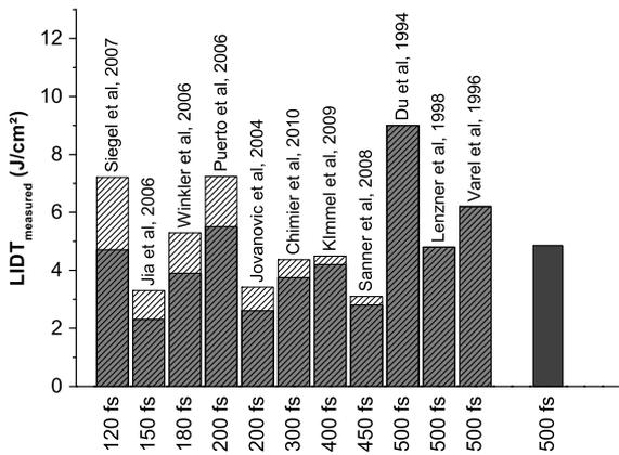
Fig. 3. Comparison of the LIDT measured by different groups on the surface of fused silica samples at 800 or 1053 nm. Measurements at the pulse duration of the experiments are given (dashed bars) and also rescaled values, with the scaling law given in the text for comparing the results at 500 fs (gray bars). Data are extracted from references [23,36–35]. The present measurement is given on the right (dark gray bar).
