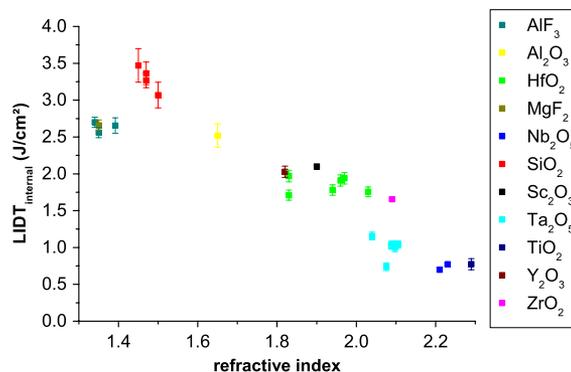
Fig. 5. Internal LIDTs of thin film materials tested in single-shot at 500 fs and 1030 nm, as a function of their refractive index at 1030 nm. This figure includes more samples than Fig. 4; i.e., samples for which the optical bandgap was not determined. See Table 2 for data and references.
