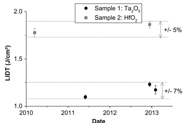
Fig. 2. Comparison of the LIDT measurements made on 2 samples ( $\text{Ta}_2\text{O}_5$  and  $\text{HfO}_2$  single layer coatings) through the years. The 2 samples have been stocked in ambient conditions, enclosed in unsealed individual polypropylene boxes between the tests.
