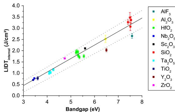
Fig. 4. LIDTs of optical thin film materials tested in single-shot at 500 fs and 1030 nm as a function of the measured optical bandgaps. The values are given as the internal LIDT, i.e., by taking into account the electric field distribution in the film. Each point corresponds to a different sample. The plain and dotted lines correspond to the plot of Eq. (3) with its error margin. See Table 2 for data and references.
