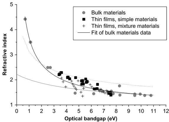
Fig. 1. Refractive indices at 1030 nm plotted as a function of optical bandgap values for the different dielectric and semiconductor samples under study. Data have been obtained from spectrophotometric measurements. The black line is a fit of bulk data. The dotted gray line is a plot of the Moss relation [20] and the solid gray line is a plot of the Herve and Vandamme relation [21].
