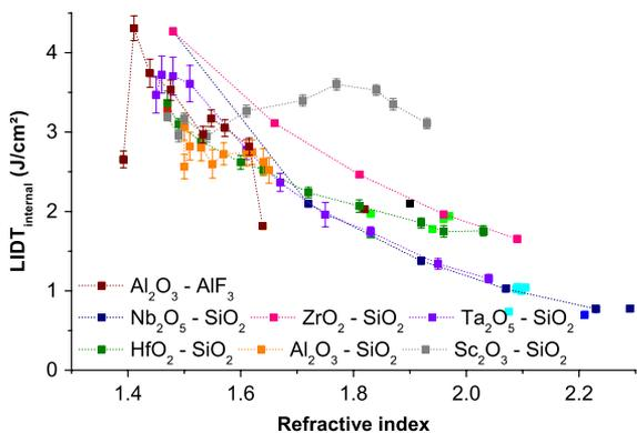
Fig. 10. Internal LIDTs of single layers of mixture materials tested under single-shot irradiation at 500 fs and 1030 nm, as a function of the refractive index at 1030 nm.
