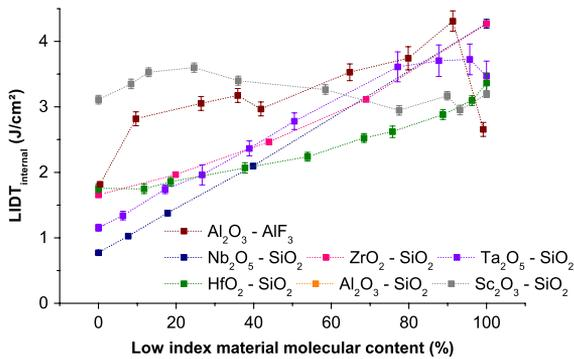
Fig. 9. Internal LIDTs of single layers of mixture materials tested under single-shot irradiation at 500 fs and 1030 nm, as a function of the low-index material molecular content. For instance, the sample 55% HfO<sub>2</sub>-SiO<sub>2</sub> should be composed of 55% of SiO<sub>2</sub> and 45% of HfO<sub>2</sub> if the film is perfectly stoichiometric. In the case of the Al<sub>2</sub>O<sub>3</sub>-AlF<sub>3</sub> samples, the low-index material is AlF<sub>3</sub>.
