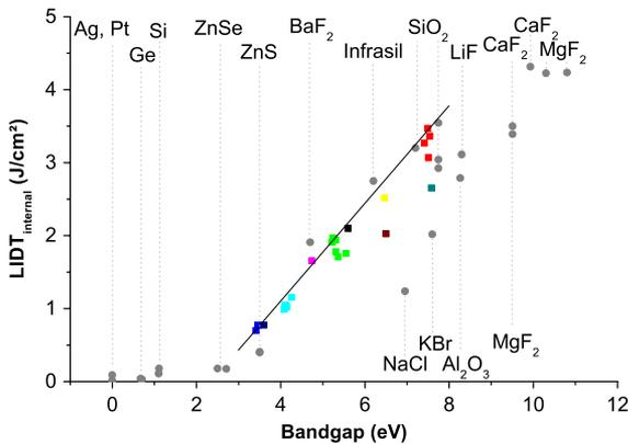
Fig. 7. LIDTs of optical thin film materials (color filled squares, with color code similar to previous figures) and bulk materials (gray filled circles) tested in single-shot at 500 fs and 1030 nm, as a function of the optical bandgaps (measured or estimated). The values are expressed as the internal LIDT. The black line is reported from Fig. 4. See Table 1 for data and references.
