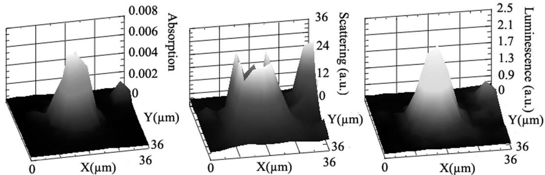
Fig. 9. Absorption, scattering, and fluorescence mappings of a micronic defect on a silica substrate. (The measurement was made with a pump beam of 6  $\mu\text{m}$  diameter; then the result on the mapping is the convolution of the beam profile with the defect.)
