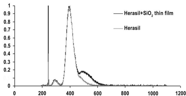
Fig. 10. Luminescence spectra of a Herasil surface and a Herasil surface coated with a  $\text{SiO}_2$  thin film, under 244 nm irradiation.
