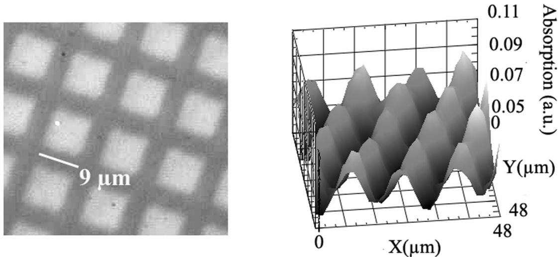
Fig. 5. (a) Nomarski image of the implanted sample. (b) Absorption mapping of the same sample (pump = 3  $\mu\text{m}$ , probe = 6  $\mu\text{m}$ ).
