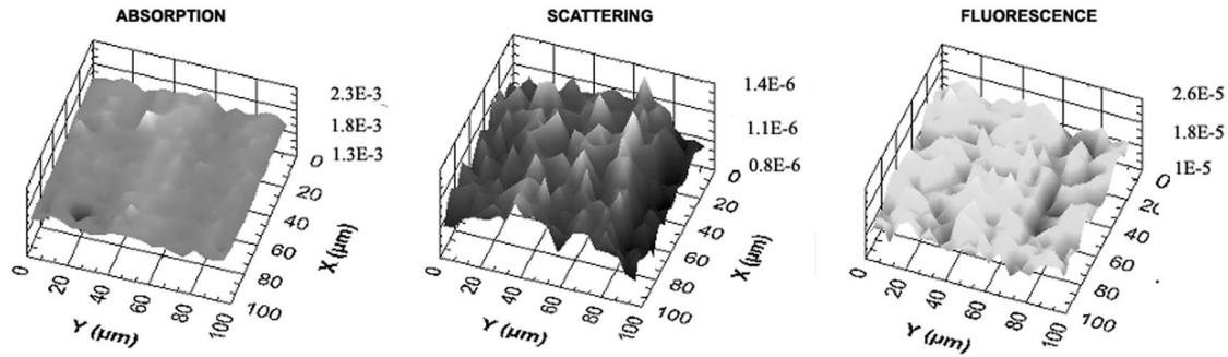
Fig. 8. Absorption, scattering, and fluorescence mappings on  $\text{HfO}_2/\text{SiO}_2$  mirrors centered at 250 nm.
