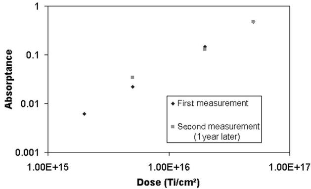
Fig. 3. Absorption measurements by spectrophotometry of ion-implanted samples.
