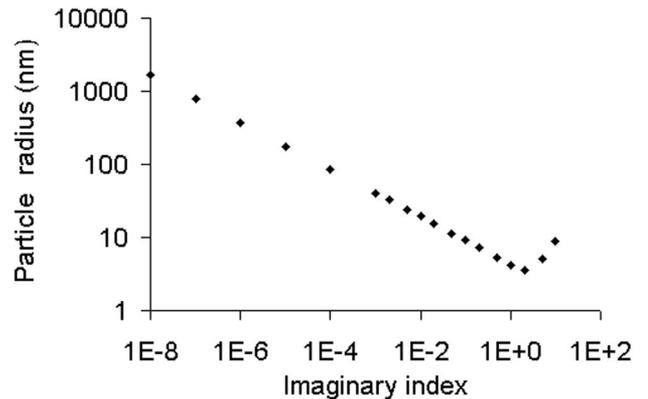
Fig. 7. Particle size as a function of its imaginary index calculated from Eq. (5) in the following conditions:  $\Delta A = 4 \times 10^{-7}$ ,  $n' = 2$ ,  $d\Phi/dS = 2.8 \times 10^{10}$ ,  $\lambda = 244$  nm,  $n_s = 1.52$ .
