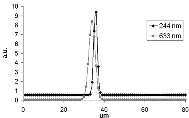
Fig. 2. Measurement of the pump- and probe-beam profiles in the plane of the sample. Case of a  $3 \mu\text{m}$  pump beam and a  $6 \mu\text{m}$  probe beam.
