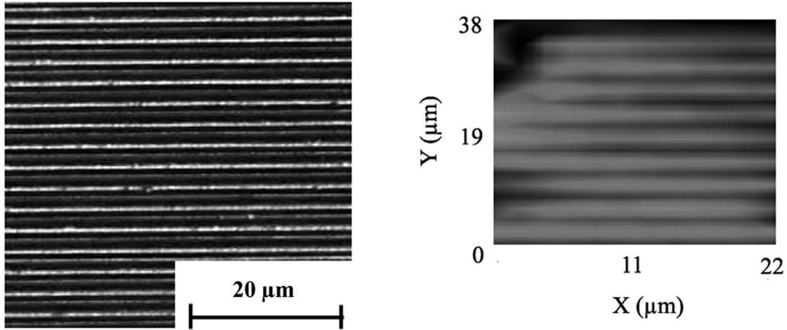
Fig. 6. (a) Nomarski image of the absorbing grating. (b) Absorption mapping of the same sample (pump = 3 μm, probe = 6 μm).
