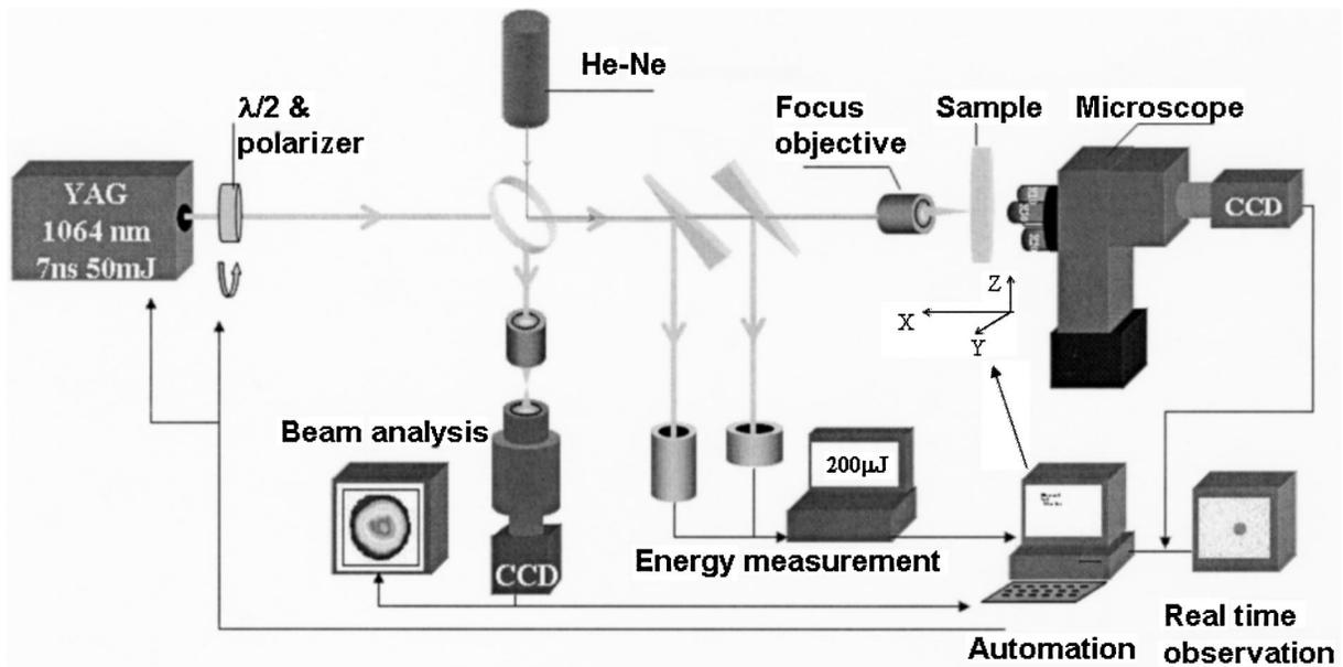
Fig. 1. Experimental setup for laser-damage testing.
