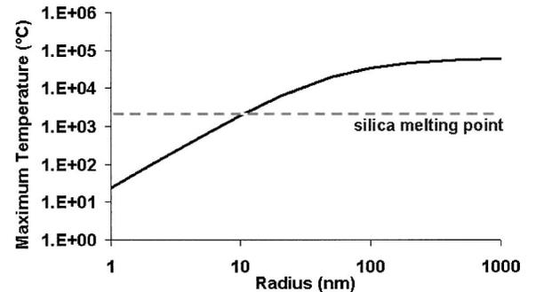
Fig. 8. Maximum temperature reached by particles embedded in silica and irradiated with an energy of  $19 \text{ J/cm}^2$  at  $1064 \text{ nm}$  during  $5 \text{ ns}$ . Dashed line, temperature of the silica melting point ( $1883 \text{ }^\circ\text{C}$ ). ( $n''\beta = 1$ .)
