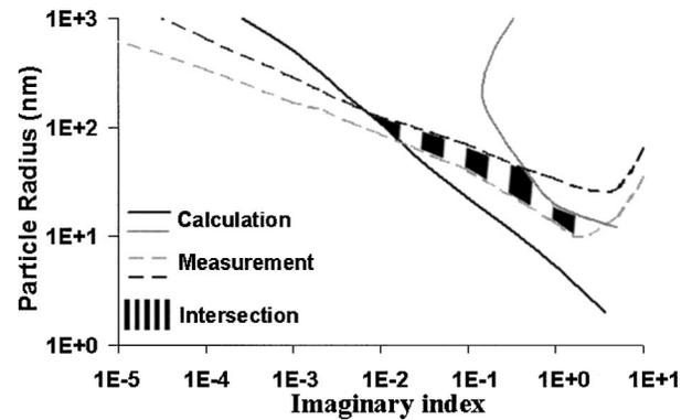
Fig. 10. Calculated and measured relationships between size and extinction index of the particle. Darker curves, lowest data; lighter curves, highest data. Striped area, intersection between thermal calculations and optical measurements, i.e., possible values of the radius and the extinction index of a laser-damage precursor embedded in silica.
