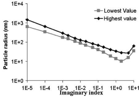
Fig. 5. Particle size as a function of extinction index, calculated from Eq. (11) for a SiO<sub>2</sub> film. Highest and lowest values are estimated from the uncertainty on  $n'$  ( $0.5 < n' < 5$ ).
