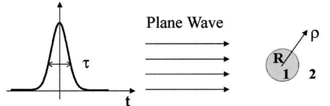
Fig. 6. Absorbing spherical particle (1) embedded in a homogenous non-absorbing medium (2) irradiated by a plane wave with a Gaussian temporal profile.
