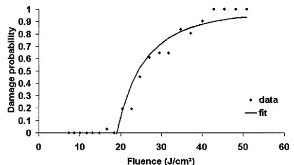
Fig. 2. Threshold curve of a silica thin film, together with fit of experimental data ( $\lambda = 1064 \text{ nm}$ ; beam diameter,  $12 \mu\text{m}$ ).
