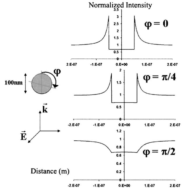
Fig. 4.  $E$ -field distribution inside and outside a 100-nm spherical particle of extinction index 1, irradiated at 1064 nm with polarization defined in this figure. The  $E$ -field distribution is represented for three polar angles in the incident plane.
