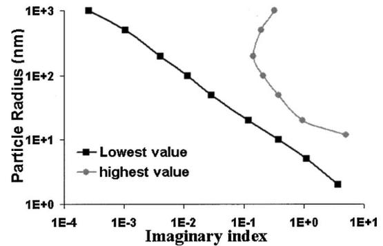
Fig. 9. Particle size as a function of extinction index, calculated from the modeling of Section 4. Highest and lowest values are estimated from the uncertainty on the different parameters (see text). Silica matrix.
