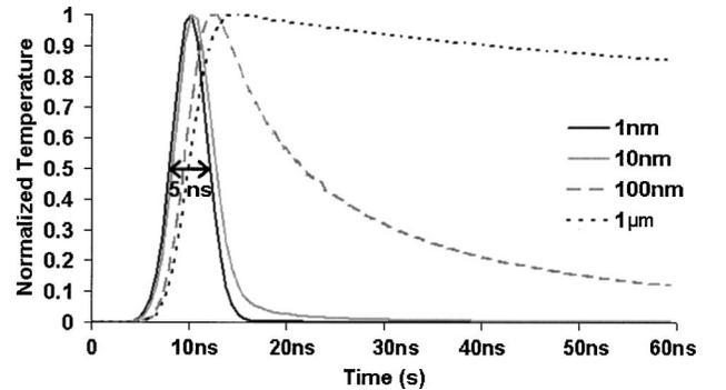
Fig. 7. Normalized temperature variations in particles embedded in silica of four diameters irradiated with an energy of  $19 \text{ J/cm}^2$  at  $1064 \text{ nm}$  during  $5 \text{ ns}$ .  $n''\beta = 1$ .
