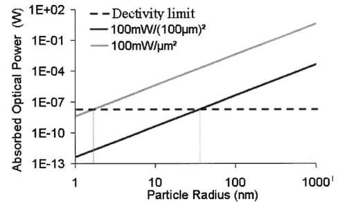
Fig. 3. Optical power absorbed by particles ( $n' = n_s$  and  $n''\beta = 1$ ) as a function of their radius. Irradiation is done with a 100-mW laser at 1064 nm, focused on a  $100\text{-}\mu\text{m}^2$  or a  $1\text{-}\mu\text{m}^2$  surface. Dashed line, average detectivity limit of photothermal measurements.
