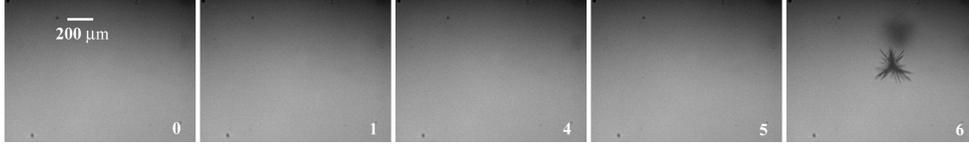
Fig. 3. Images after successive shots in the bulk of a Suprasil glass at  $110J/cm^2$ . Damage appears after the 6th shot, without any visible modification on the previous shots.
