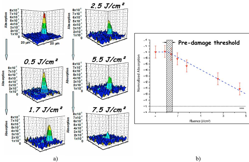
**Fig. 4.** Pre-damage stage for 250 nm-gold inclusions. a) Evolution of HRPD images of 250 nm-gold inclusions after one shot at the given fluence (from 0.5 to 7.5 J/cm<sup>2</sup>). b) Evolution of the gold inclusion absorption under single shot irradiation, deduced from HRPD images.
