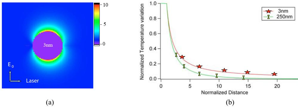
**Fig. 2.** (a) Example of calculation of the normalized E-field distribution inside and outside a 3-nm spherical gold inclusion embedded in silica irradiated at 1064 nm with polarization described in figure. This calculation is performed in the plane of incident field, thanks to Mie theory. (b) Normalized modulated temperature distribution inside and outside the inclusion versus normalized distance for two diameters 3 and 250 nm and for modulation frequency  $10^6$  Hz.
