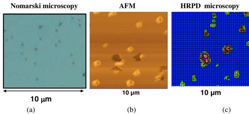
**Fig. 5.** Case of gold inclusions of diameter 3 nm inserted at a depth of 30 nm with an area density of 1 incl./ $\mu\text{m}^2$ . Observation of the damages on the surface by using three different microscopes: Nomarski (a), atomic force (b) and photothermal deflection (c). We observe the small increase of absorption in the flaked regions showing the modification of the surrounding silica.
