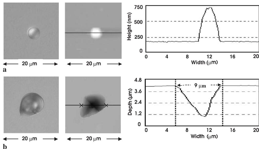
**FIGURE 5** Nomarski microscope image and AFM scan of the same surface of our  $2\text{-}\mu\text{m}$ -thick upper film sample, showing **a** the dome situated above a gold inclusion and **b** the crater formation after irradiation. Plots of vertical heights vs. horizontal distances show dome and crater profiles
