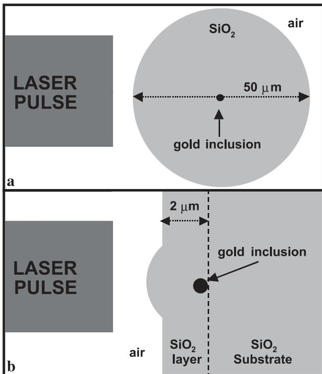
**FIGURE 1** Configurations of two different geometries studied in this work, both with gold spheres of 600-nm diameter: **a** the inclusion is embedded in a spherical bulk silica substrate, **b** the inclusion is deposited on a thin silica film deposited on a bulk silica substrate, and is then covered by a second silica thin film
