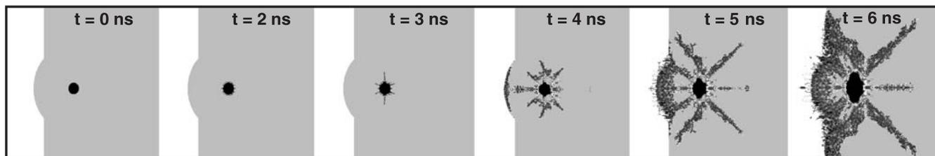
**FIGURE 4** Simulation of the fracture propagation produced by irradiation of the gold inclusion located near a free surface, at different times following the arrival of the laser pulse. The fluence is  $6 \text{ J/cm}^2$ , the wavelength  $355 \text{ nm}$  and the pulse duration  $3 \text{ ns}$  FWHM
