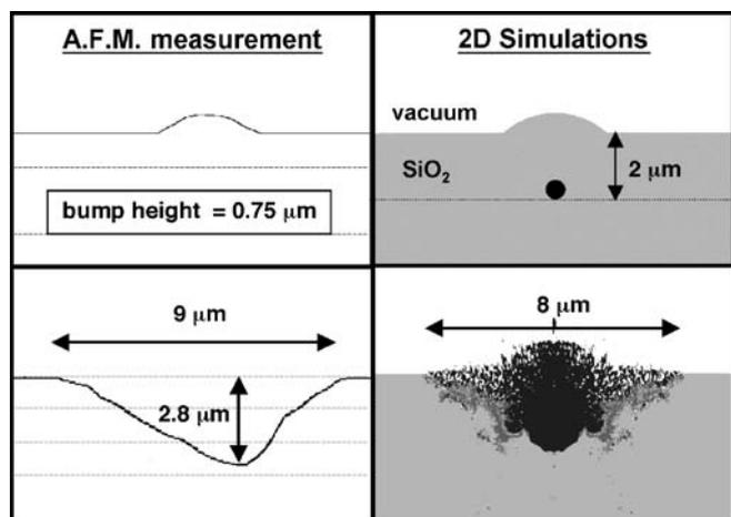
**FIGURE 6** Comparison of AFM measurements and code HESIONE simulations for an inclusion at depth  $2 \mu\text{m}$ . The *upper part* shows the initial configuration, while the *lower part* corresponds to damage produced by laser irradiation ( $6 \text{ J/cm}^2$ ,  $355$  nm). The simulation indicates the vertical velocity field a few ns after the end of the pulse
