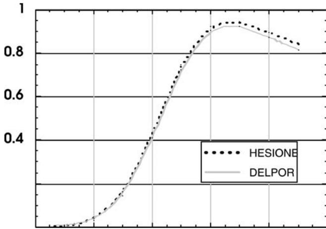
**FIGURE 2** The pressure in the gold inclusion as a function of time  $t$  in the laser pulse, as calculated by the 1-D code DELPOR (solid curve) and the 2-D code HESIONE (dashed curve), for a fluence of  $0.1 \text{ J/cm}^2$
