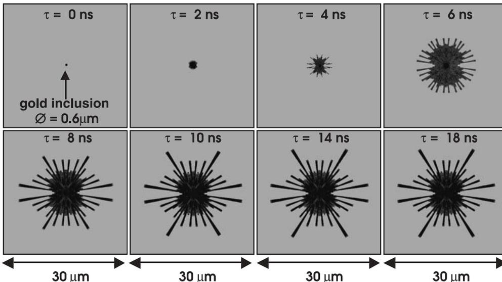
**FIGURE 3** Simulation of stresses in bulk silica, at different times, produced by laser irradiation of a gold sphere of radius 600 nm. The fluence is  $6 \text{ J/cm}^2$ , the wavelength 355 nm and the pulse duration 3 ns FWHM
