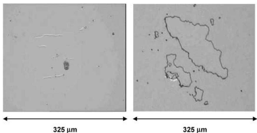
**FIGURE 3** Nomarski microscope images of site damage produced at a laser fluence of 4.2 J/cm<sup>2</sup> for samples containing gold nanoparticles: (left) density of 10 nanoparticles/ $\mu\text{m}^2$ , (right) density of 100 nanoparticles/ $\mu\text{m}^2$
