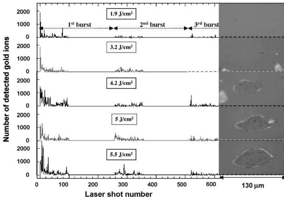
**FIGURE 12** The number of gold ions detected as a function of shot number for the first 100 shots of three consecutive bursts on the same site at the fluences indicated. On the *right* are shown corresponding Nomarski microscope photographs of the damaged sites after receiving three bursts of 256 shots
