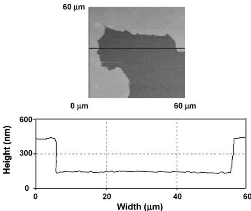
**FIGURE 4** AFM observation of a severely damaged site produced at a laser fluence of 4.2 J/cm<sup>2</sup>. The upper part shows a zone where deep surface excavation has occurred. The lower part shows the profile along the horizontal line indicated
