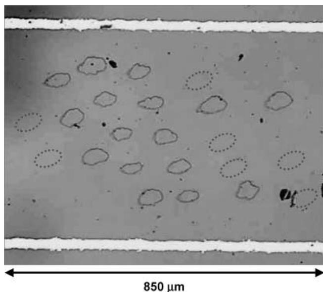
**FIGURE 6** Nomarski photograph of the principal irradiated zone on a sample. Each damage site corresponds to one burst of 256 shots. Some sites, where no damage was observed, are indicated by *dashed ellipses*. The chromium strips used to evacuate any charge on the sample are clearly visible
