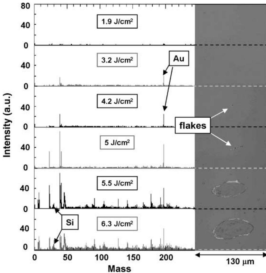
**FIGURE 8** Six mass spectra (obtained at the fluences indicated) and the corresponding Nomarski microscope photographs of the damage produced by the burst of 256 shots. Each spectrum corresponds to a fresh site
