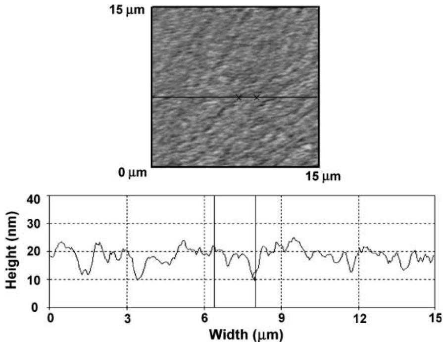
FIGURE 2 AFM image of a sample showing surface rugosity (upper). Details of a cut along the horizontal line, which furnishes an estimation of the mean surface rugosity (lower)
