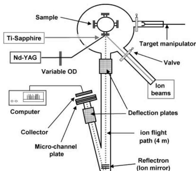
FIGURE 5 Schematic picture of the time-of-flight mass spectrometer
