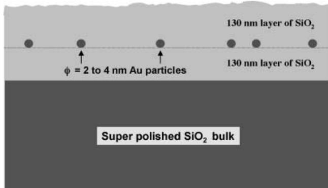
FIGURE 1 Figurative drawing of a section of a sample
