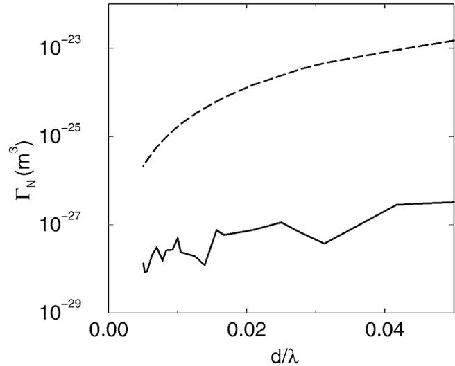
FIG. 2. Study of the normalized optical torque vs  $d/\lambda$  on a dielectric sphere ( $\varepsilon=2.25$ ) with radius  $a=\lambda/4$  illuminated by a circularly polarized plane wave. Solid line the optical torque is computed in using Eq. (7), and dashed line without taking into account the radiative reaction term in Eq. (7).
