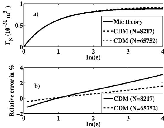
FIG. 3. Study of the normalized optical torque on a sphere with radius  $a = \lambda/4$  illuminated by a circularly polarized plane wave. (a) Optical torque vs  $\text{Im}(\varepsilon)$  [ $\text{Re}(\varepsilon)=2.25$ ] obtained from the Mie series (plain line), and the CDM:  $N=8217$  (dashed line), and  $N=65752$  (dotted line). (b) Relative error in percent for optical torque obtained from the Mie series and from the CDM.
