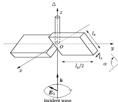
FIG. 5. The object under study is a micropropeller illuminated by a right-handed circularly polarized wave which propagates along the  $z$  axis:  $\mathbf{E}_0 = E_0(1, i, 0)e^{ik_0z}$ . The angle between the two vanes and the  $x$  axis is  $\alpha$ .
