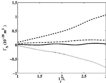
FIG. 6. The object under study is a micropropeller (Fig. 5) illuminated by a circularly polarized plane wave. The normalized optical torque is plotted vs  $l_y$  with  $l_x=0.8\lambda$ ,  $l_z=0.4\lambda$  for different angles  $\alpha$ :  $\alpha=0^\circ$  in plain line,  $\alpha=60^\circ$  in dashed line,  $\alpha=90^\circ$  in dot-dashed line, and  $\alpha=-60^\circ$  in dotted line.
