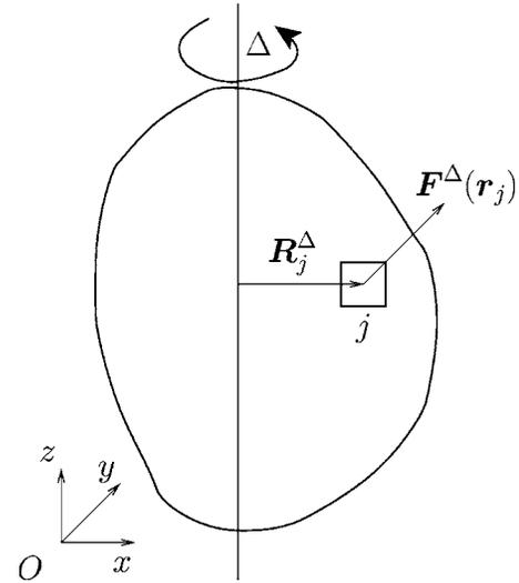
FIG. 1. Arbitrary object with a rotation axis of  $\Delta$ . The square is an element of the discretization of the object.  $\mathbf{R}_j^\Delta$  is the distance between subunit  $j$  and the rotation axis, and  $\mathbf{F}^\Delta(\mathbf{r}_j)$  is the component of the optical force perpendicular to the axis  $\Delta$  acting on subunit  $j$ .
