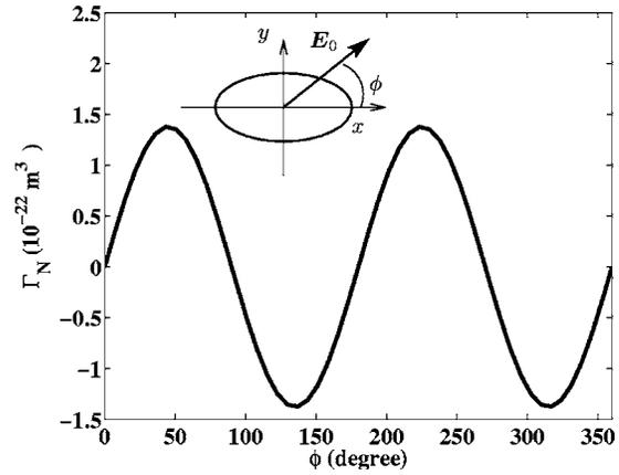
FIG. 4. Normalized optical torque vs  $\varphi$  the angle between the  $x$  axis and  $\mathbf{E}_0$ . The object is an ellipsoid wider in the direction of  $x$ , see inset.
