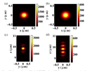
Fig. 2. (Color online) Global PSF of an ISO microscope, simulated for two different objectives in air: (a) and (c) ideal objective with NA =  $\sin\theta_{\rm max}=0.99$ ; (b) and (d) realistic objective, NA =  $\sin\theta_{\rm max}=0.80$ . These images corresponds to slices taken in the (a), (b) transverse and (c), (d) axial planes.
