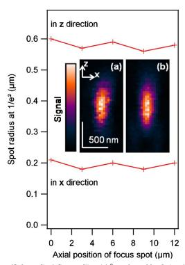
Fig. 9. (Color online) Spot radii at  $1/e^2$ , evaluated by fitting (with a Gaussian curve) axial and transverse profiles taken from fluorescence images of a 100 nm bead, measured while controlling the actual plane where light focuses using the SLM. Insert: axial slices of two of these images, measured while focusing (a) in the genuine focal plane of the lens and (b) in a plane located  $12\,\mu\mathrm{m}$  before it.
