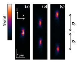
Fig. 10. (Color online) Fluorescence images (axial slices) of a 100 nm bead, measured with time-reversal phase masks that yield pairs of spots separated by (a) 0, (b) 2, and (c)  $4\,\mu$ m along the optical axis in the absence of the mirror.
