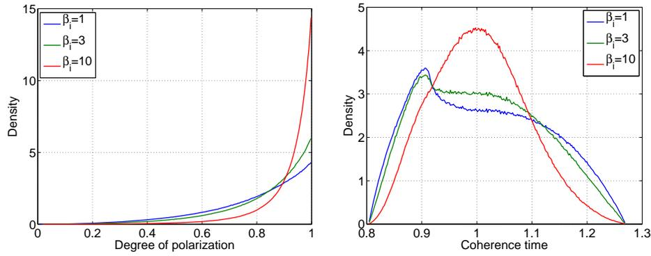
Fig. 2. Densities of the degree of polarization (left) and coherence time (right) for parameters  $\mu_i = 1/2$ ,  $\theta = \pi/8$ ,  $r \simeq 1.8$  and three values of parameter  $\beta_i$ .
