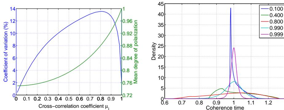
Fig. 3. The coherence time coefficient of variation and the mean DOP against the cross-correlation coefficient (left) and densities of the coherence time for several values of the cross-correlation coefficient (right) for parameters  $\beta_i = 1$  and  $\theta = \frac{\pi}{4} \mu_i$ .
