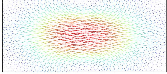
**Fig. 2.** Transverse component of the electric field for a resonance mode of angular frequency  $\omega c = 3.78m$  ( $\beta = 0$ ) in an helicoidal metallic structure of rectangular cross-section (thickness =  $1.02m$ , length =  $2.29m$ , torsional parameter  $\alpha = 1m^{-1}$ ). The picture suggests that the twist confines the resonant mode within the disc inscribed into the rectangular cross-section.
