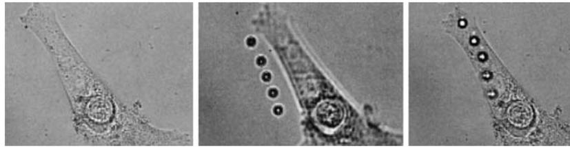
**Fig. 9** A set of five latex beads of diameter 5  $\mu\text{m}$  are extracted from the confinement chamber and put into contact with a selected COS-7 cell (*left*). The traps pattern was defined via the
