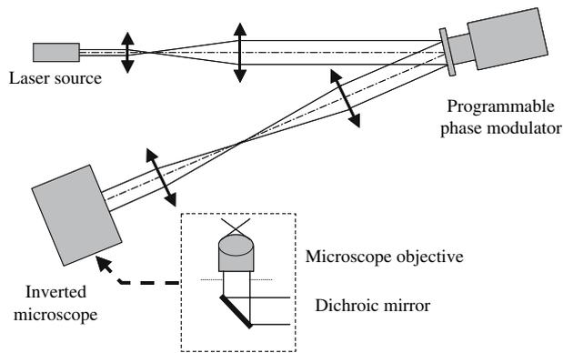
**Fig. 1** Scheme of the HOT setup (*top view*)
