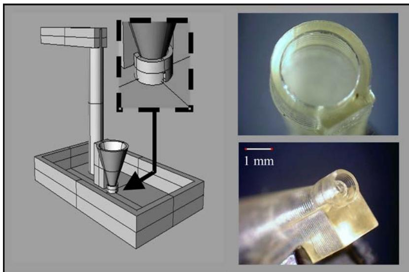
Brussels, Belgium) and 30% with 1,6-hexanediol diacrylate (HDDA, UCB Chemicals). With such a material, the fabrication rate is of two layers per minute, with a 800 ms exposure time of each frame for layers  $50\ \mu\text{m}$  thick.
