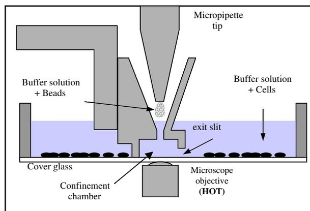
**Fig. 6** Once fabricated, the reservoir is applied on a commercially available chambered coverglass. Once the beads are deposited on the coverglass, we use H<sub>2</sub>O<sub>2</sub> to trap beads inside the confinement chamber. Then the sample is moved thanks to programmable stages, in order for the beads to pass through the exit slit and get onto the target cell. The reservoir is permanently placed inside the sample and never removed during the experiment
