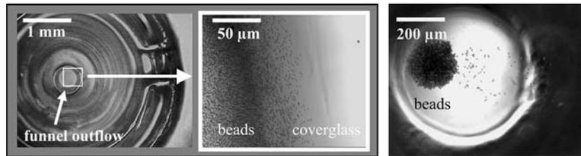
**Fig. 7** Beads dispersion on the microscope cover glass placed under the funnel outflow. One can confirm the limited diffusion of beads on the glass, and hence demonstrate the ability of the
