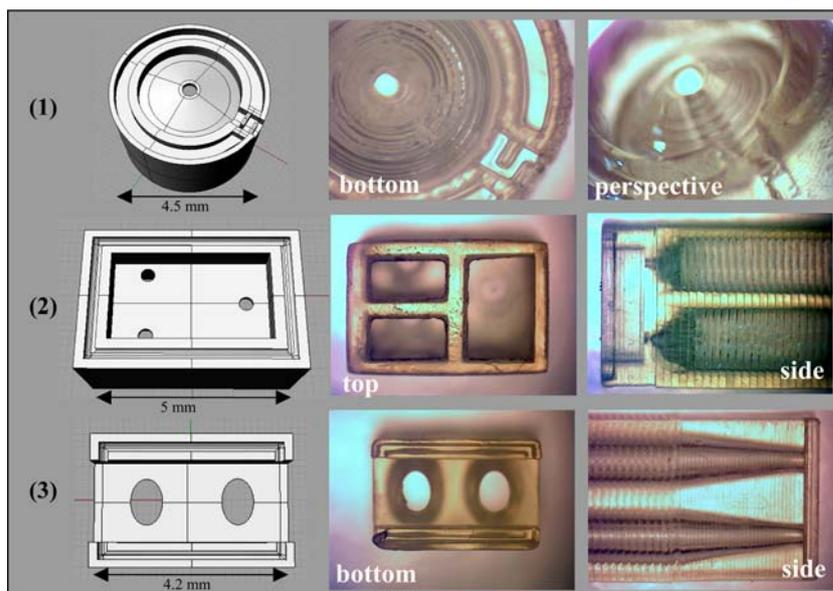
**Fig. 5** A specific reservoir structure to keep beads and cells separated in a liquid sample composed of 75 layers, each one of thickness  $100\ \mu\text{m}$
