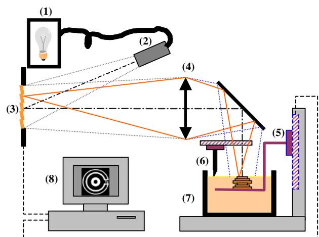
**Fig. 2** Scheme of the  $\mu\text{SL}$  setup. (1) High-pressure Hg–Xe light source; (2) uniform illumination lens; (3) dynamic mask; (4) projection/reduction lens; (5) vertical moving stage; (6) scraper; (7) bath of liquid resin; (8) personal computer
