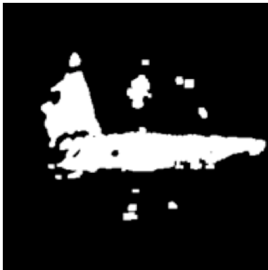
Fig. 9. Fake gun concealed by a leather jacket: combination of the result obtained with combined H and V polarizations
