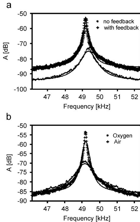
Fig. 6. The effect of feedback for different working media. (a) In air and (b) in air and oxygen.
