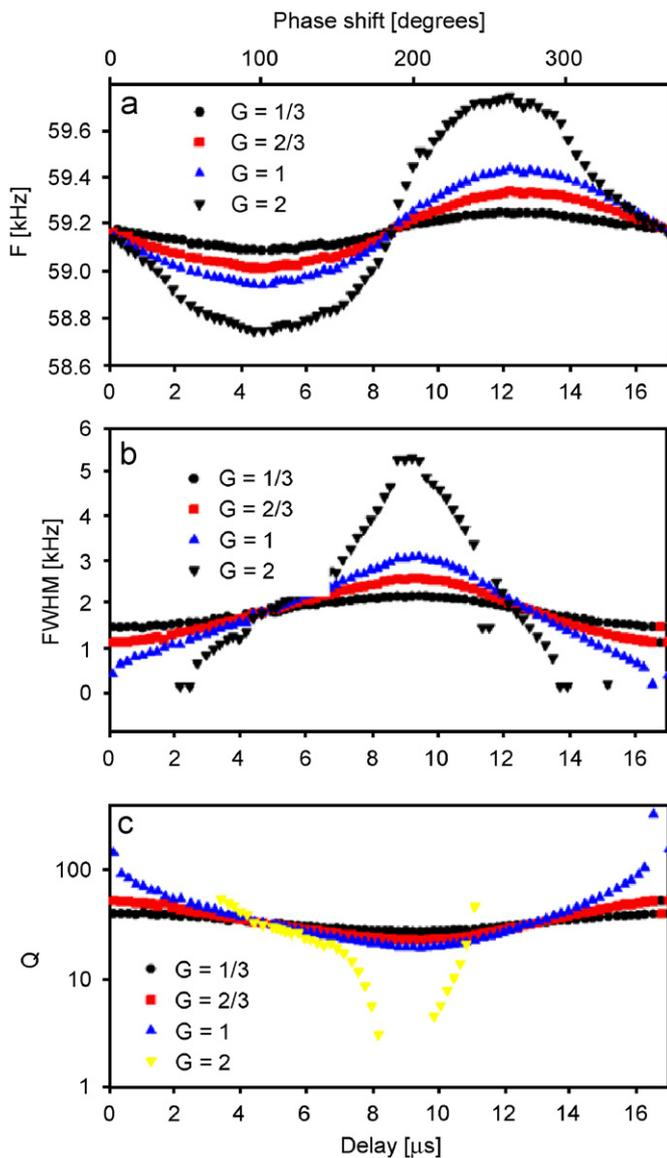
Fig. 3. The variation of resonant frequency, FWHM, and  $Q$  factor with varied delay while different gains were applied. (a) Resonant frequency, (b) FWHM, and (c)  $Q$  factor.
