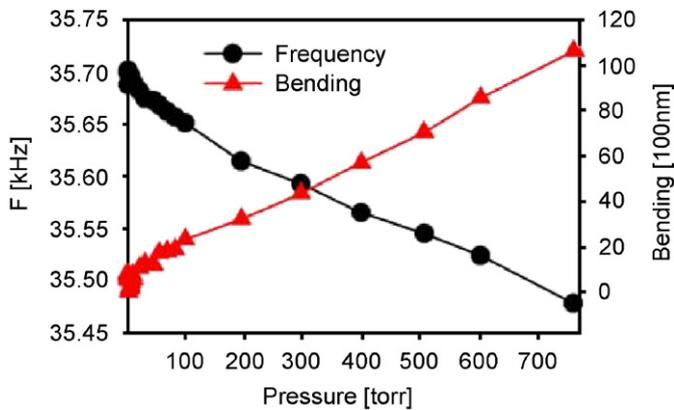
Fig. 5. The change of the resonance frequency and bending of a microcantilever with varying air pressure.
