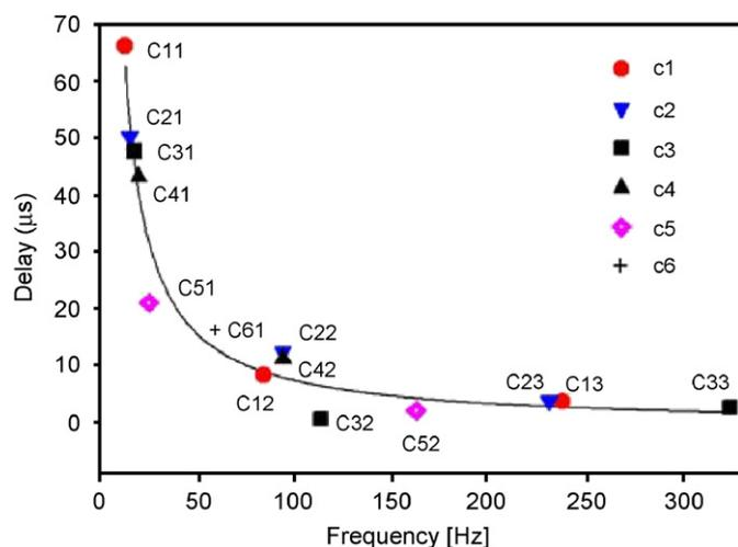
Fig. 8. The response time required by the cantilever for different resonant frequencies. The solid line is the inverse first order fit curve.
