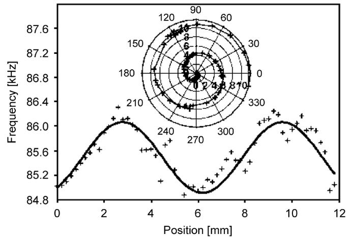
Fig. 7. Frequency response and phase shift of the second resonance peaks (85 kHz) for a delayed-feedback system. The lower part shows the frequency shift while the cantilever is traveling toward the acoustic transducer. The solid curve is the sinusoidal fit. The upper part shows the corresponding phase shift of the cantilever during its travel.
