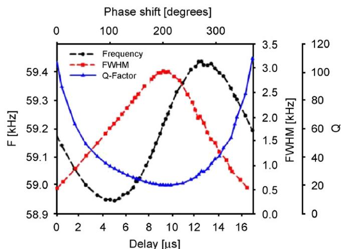
Fig. 2. The shift of resonant frequency, FWHM, and  $Q$  factor as a result of varied delay. Here the system delay is also represented in the form of phase shift.
