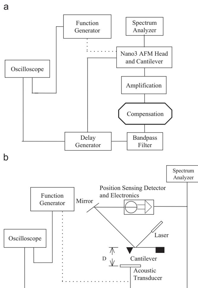
Fig. 1. Schematic of the experimental setup. In setup (a), delay modules are used to generate system delay and an internal piezoelectric actuator is used as the cantilever oscillator. In setup (b), the delay modules and the piezoactuator are replaced by an acoustic transducer.
