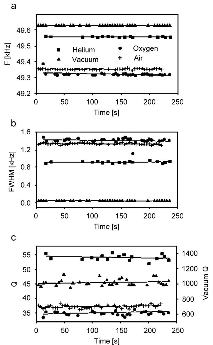
Fig. 4. The room temperature environmental effect on the noise parameters, frequency  $F$ , FWHM, and quality factor  $Q$  detected at the fundamental frequency of the microcantilever. In (a) the fundamental frequency, in (b) FWHM, and in (c) the quality factor are monitored in four distinct environments, air, oxygen, helium, and vacuum. The solid curves are linear fits.
