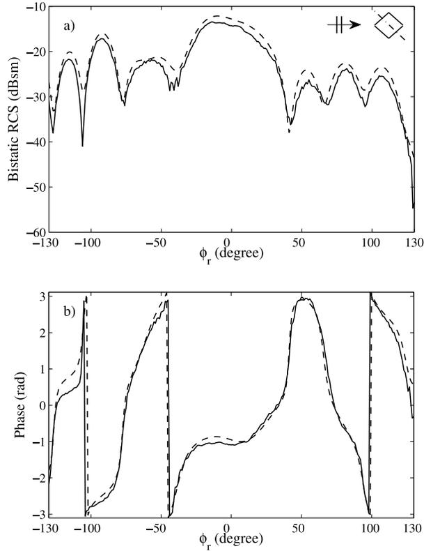
**Figure 10.** Comparison of (a)  $|E_{d,\theta\theta}|$  and (b)  $\arg(E_{d,\theta\theta})$ , measured (full line) and simulated (dashed line). This result is obtained for the Ertalon cylinder at 8 GHz and for  $\phi_s = 60^\circ$  and  $\phi_o = 45^\circ$  ( $\mathcal{F}_{\theta\theta} = 0.047$ ).
