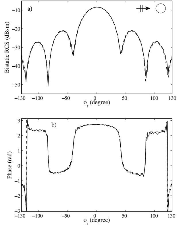
**Figure 5.** Comparison of (a)  $|E_{d,\theta\theta}|$  and (b)  $\arg(E_{d,\theta\theta})$ , measured (full line) and simulated (dashed line). This result is obtained for the Altuglass sphere at 8 GHz and for  $\phi_s = 90^\circ$  ( $\overline{\mathcal{F}_{\theta\theta}} = 0.002$ ).
