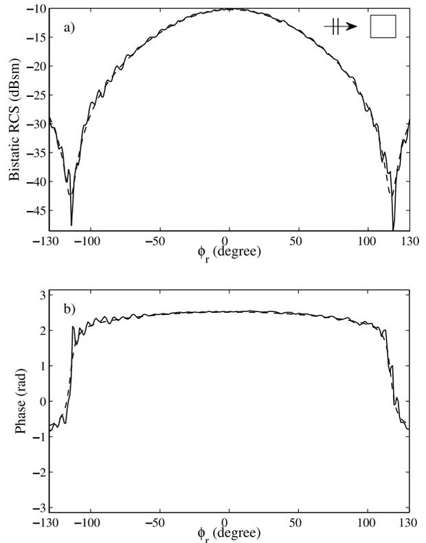
**Figure 6.** Comparison of (a)  $|E_{d,\theta\theta}|$  and (b)  $\arg(E_{d,\theta\theta})$ , measured (full line) and simulated (dashed line). This result is obtained for the Polyethylene cube at 2 GHz and for  $\phi_s = 90^\circ$  and  $\phi_o = 0^\circ$  ( $\mathcal{F}_{\theta\theta} = 0.001$ ).
