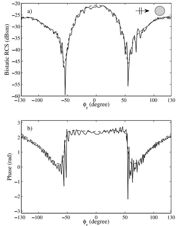
**Figure 3.** Comparison of (a)  $|E_{d,\theta\theta}|$  and (b)  $\arg(E_{d,\theta\theta})$ , measured (full line) and simulated (dashed line). This result is obtained for the metallic sphere at 8 GHz and for  $\phi_s = 30^\circ$  ( $\mathcal{F}_{\theta\theta} = 0.029$ ).
