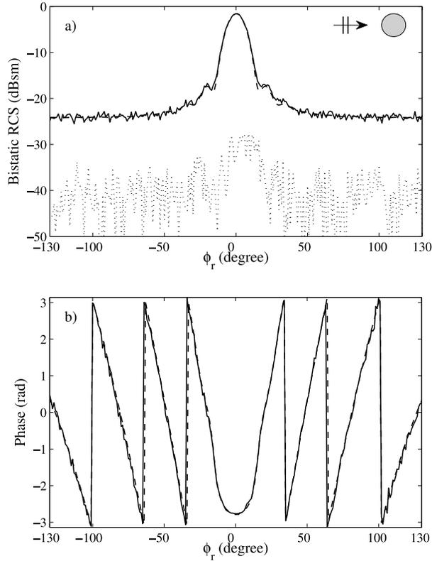
**Figure 2.** Comparison of (a)  $|E_{d,\theta\theta}|$  and (b)  $\arg(E_{d,\theta\theta})$ , measured (full line) and simulated (dashed line).  $|E_{d,\theta\varphi}|$  is also plotted in dotted line in Figure 2a to show the magnitude difference. This result is obtained for the metallic sphere at 18 GHz and for  $\phi_s = 90^\circ$  ( $\mathcal{F}_{\theta\theta} = 0.004$ ).
