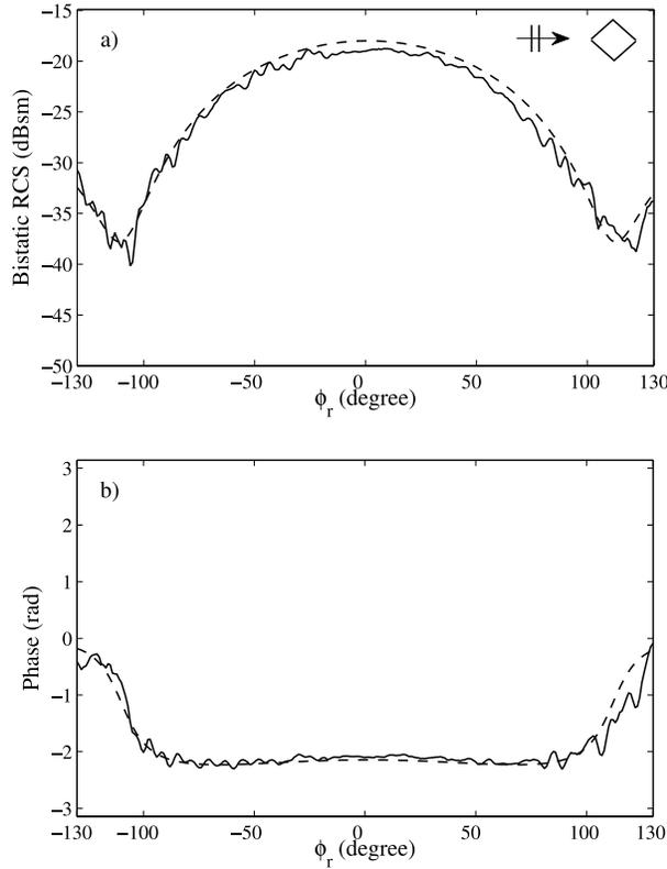
**Figure 7.** Comparison of (a)  $|E_{d,\theta\theta}|$  and (b)  $\arg(E_{d,\theta\theta})$ , measured (full line) and simulated (dashed line). This result is obtained for the Polyethylene cube at 2 GHz and for  $\phi_s = 30^\circ$  and  $\phi_o = -45^\circ$  ( $\mathcal{F}_{\theta\theta} = 0.013$ ).
