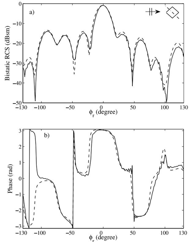
**Figure 9.** Comparison of (a)  $|E_{d,\theta\theta}|$  and (b)  $\arg(E_{d,\theta\theta})$ , measured (full line) and simulated (dashed line). This result is obtained for the Ertalon cylinder at 8 GHz and for  $\phi_s = 90^\circ$  and  $\phi_o = 45^\circ$  ( $\mathcal{F}_{\theta\theta} = 0.026$ ).
