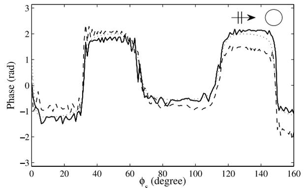
**Figure 12.**  $\arg(E_{a,\theta\theta})$  for a source moving on the arch. This result is obtained for the Altuglass sphere at 11 GHz and for  $\phi_o = \phi_r = 0^\circ$ . Dashed line: measured with a target presumably positioned at  $O$  ( $\mathcal{F}_{\theta\theta} = 0.100$ ). Full line: measured with a target positioned 2.3 mm below the previous position ( $\mathcal{F}_{\theta\theta} = 0.047$ ). Dotted line: simulated with the target centered at  $z = 0.0$  mm.
