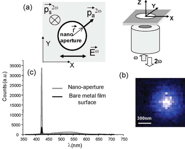
Fig. 1. (Color online) (a) Nonlinear induced dipoles in a metal nanoaperture. (b) Experimental scheme of the nonlinear microscopy imaging and SHG image of a circular nanoaperture (diameter 195 nm). (c) Emission spectrum from a nanoaperture and the bare metal surface, measured using a spectrograph at the exit of the microscope (diameter 195 nm, excitation: horizontal polarization). Typical average power at the objective focus: a few milliwatts.
